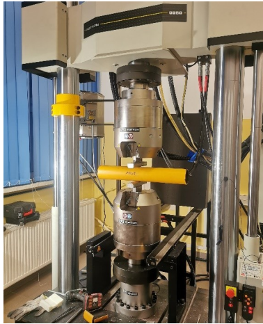
Fig. 22. Instron 8850 machine with tested sample
