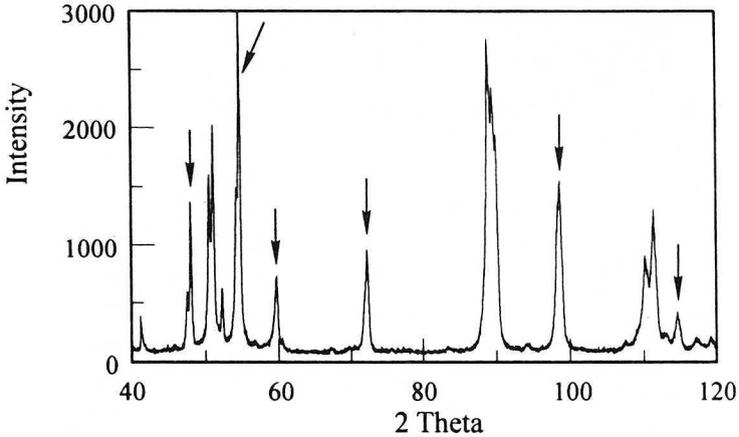
Fig. 4. X-ray spectrum of the sample aged for 4000 hours, cold rolled to 70% reduction and annealed at 650°C for 1000 hours; peaks from the  $\text{Ni}_3\text{Mo}$  phase are marked by arrows
