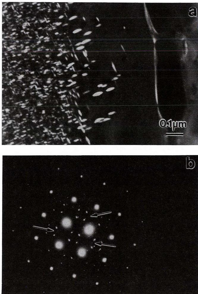
Fig. 9(a). Dark field image of a zone denuded of ordered domains around grain boundary precipitates, (b) corresponding SAD pattern; arrows show SRO reflections
