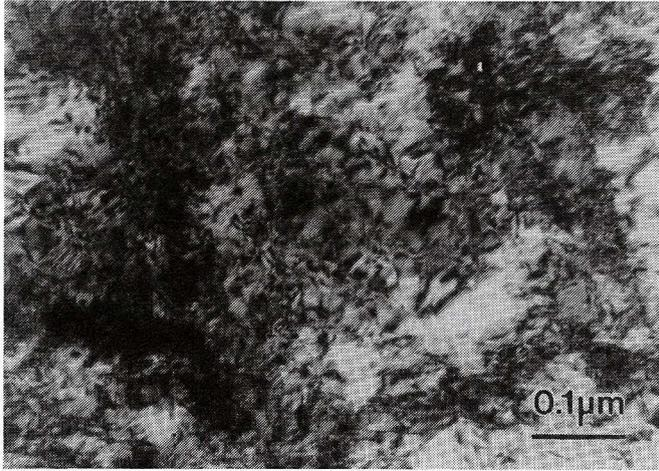
Fig. 17. The dislocation structure in a grain with the Goss orientation; deformation 70%, sample aged for 4000 hours
