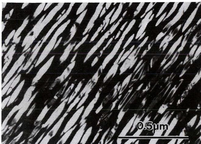
Fig. 3. Dark field image of the ordered domains after aging at 650°C for 4000 h
