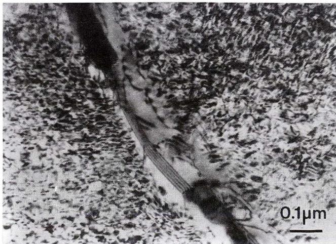
Fig. 8. Typical precipitates on a grain boundary in a sample subjected to the intermediate heat treatment
