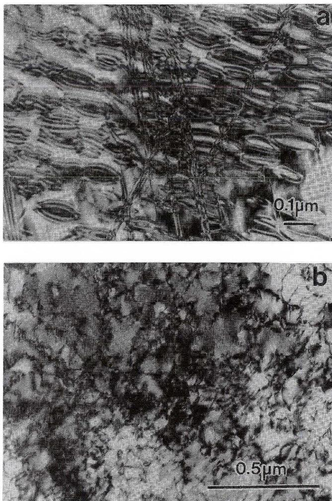
Fig. 13. Typical microstructure in samples deformed to failure: a) at 750°C (ordered precipitates, mechanical twins, b) at 775°C (no precipitates, dislocations)
