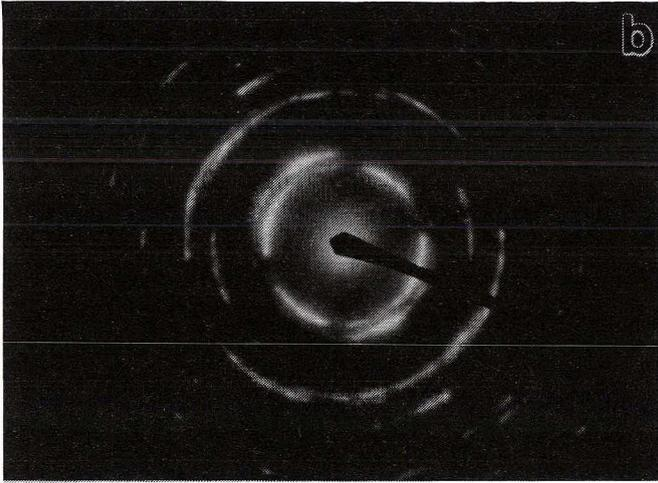
Fig. 18. Shear bands in a sample deformed to 70% by rolling; sample aged for 4000 hours (a) and corresponding SAD pattern (b)
