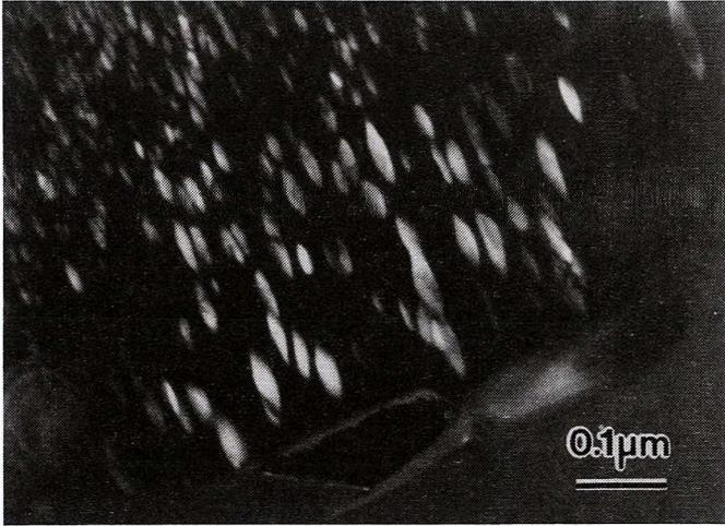
Fig. 10. A microphotograph illustrating how the long-range domain size changes with the distance from a grain boundary; dark field image
