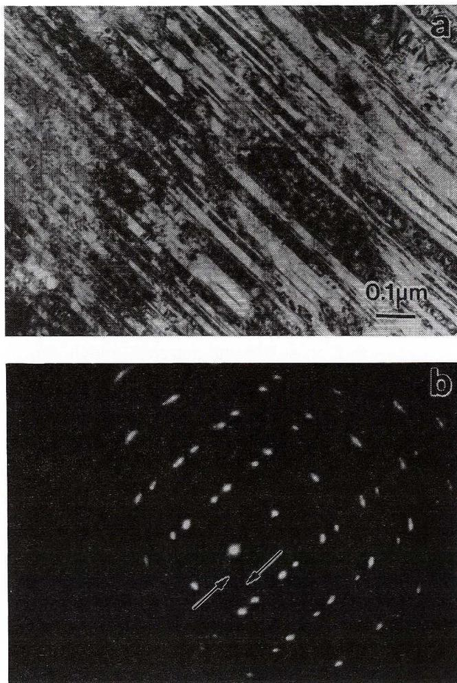
Fig. 16. Typical deformation twins in sample aged for 4000 hours and subjected to rolling with 70% reduction in thickness (a); the SAD pattern (b) shows extra spots from the  $\text{Ni}_2(\text{Mo,Cr})$  phase
