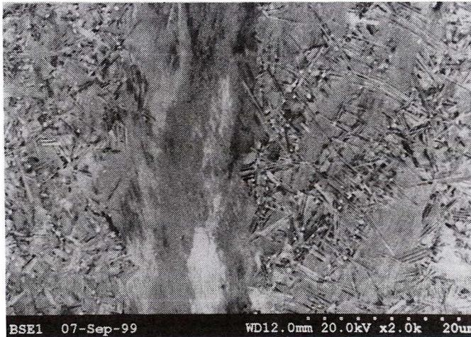
Fig. 5. SEM backscattered image of the microstructure of the conventionally aged then cold rolled sample to 80% reduction and subsequently annealed at 650°C for 1000 hours
