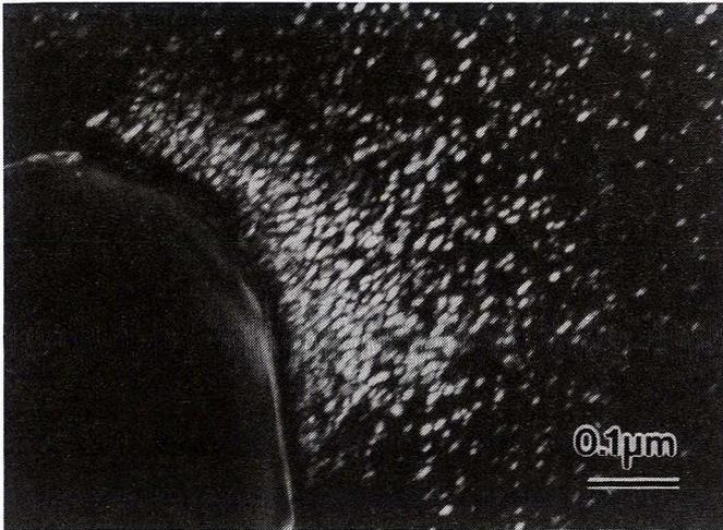
Fig. 11. Increased density of ordered phase domains close to a big particle in samples after aging of intermediately heat treated sample at 980°C
