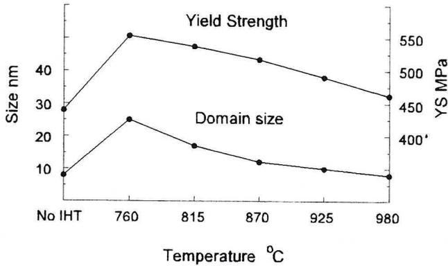
Fig. 7. Dependence of the ordered particles' size and the yield strength of the alloy on the IHT temperatures
