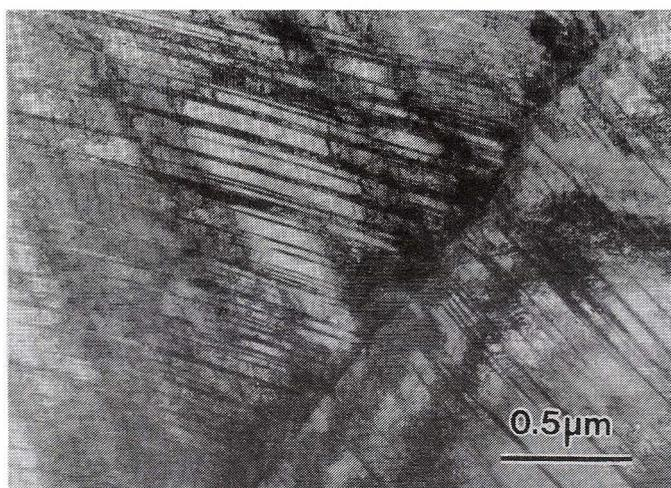
Fig. 15. Typical deformation twins in conventionally aged sample tensile tested at room temperature
