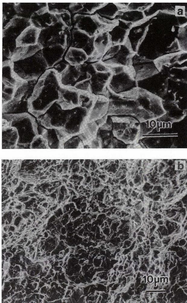
Fig. 12. Typical fracture surfaces in the specimen aged for 4000 h and deformed at 650°C: a) area close to the free surface, b) area close to the center
