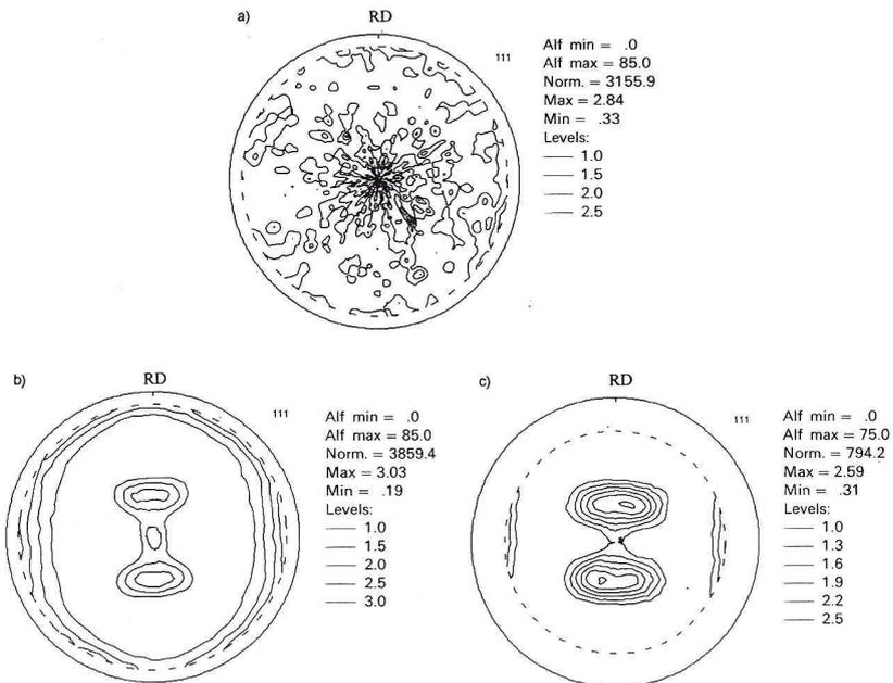
Fig. 19.  $\{111\}$  pole figures for a) undeformed sample, b) after 80% deformation of unaged sample, c) after 70% deformation for the sample aged for 4000 hours
