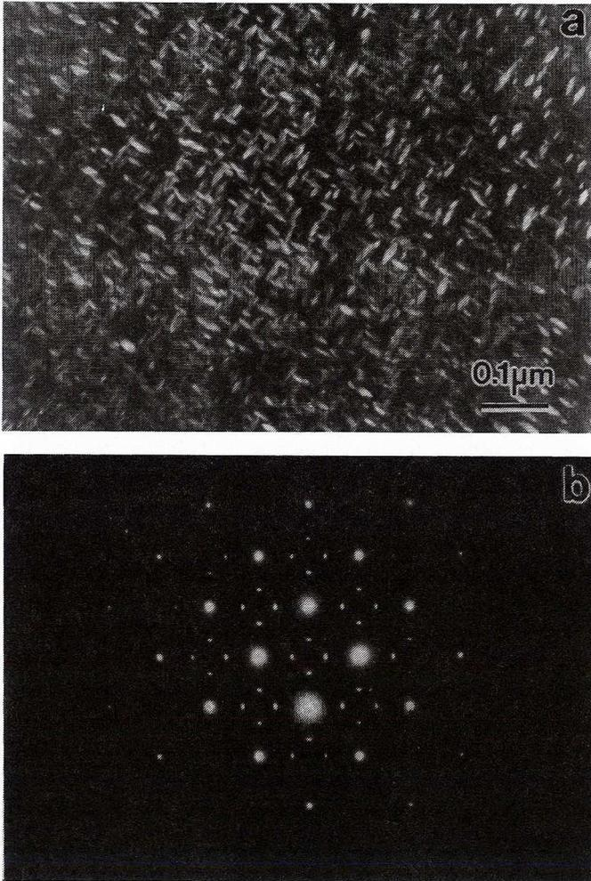
Fig. 1a. Typical Dark Field image of the ordered particles, (b) corresponding SAD pattern. (A relatively large objective aperture used in the dark field procedure allowed all four reflections from the ordered phase to contribute to the image of four, out of six possible, sets of the particles' orientations)
