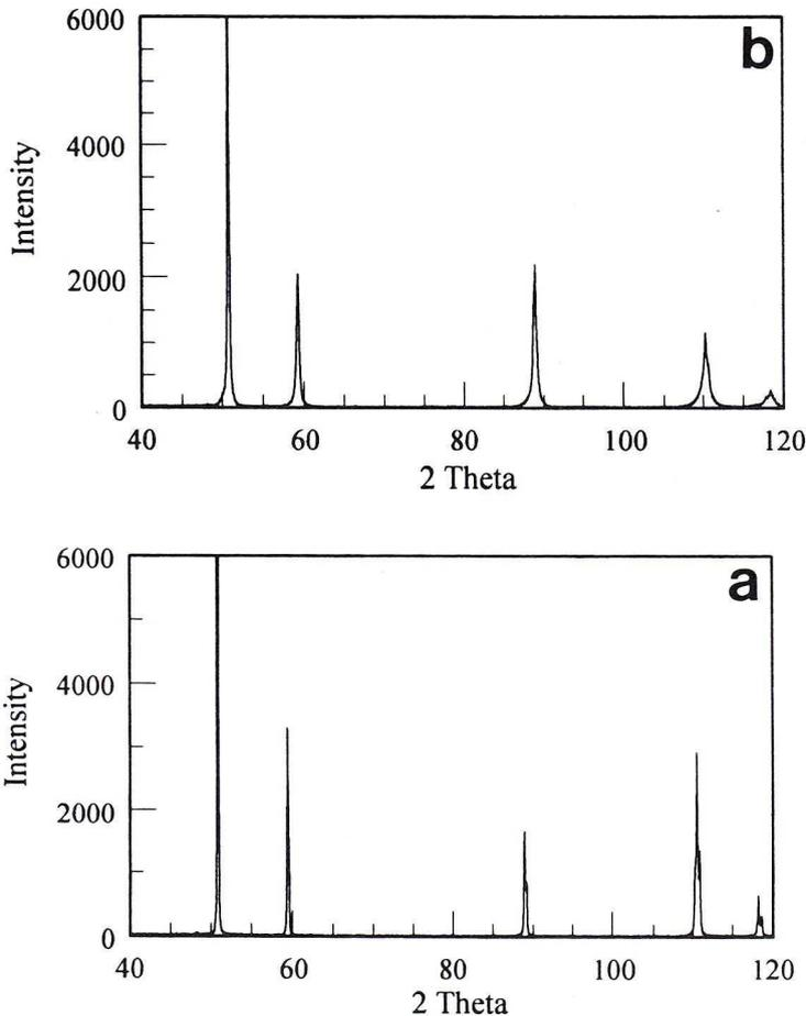
Fig. 2. X-ray spectra of selected samples: a) annealed material, b) conventionally heat treated material
