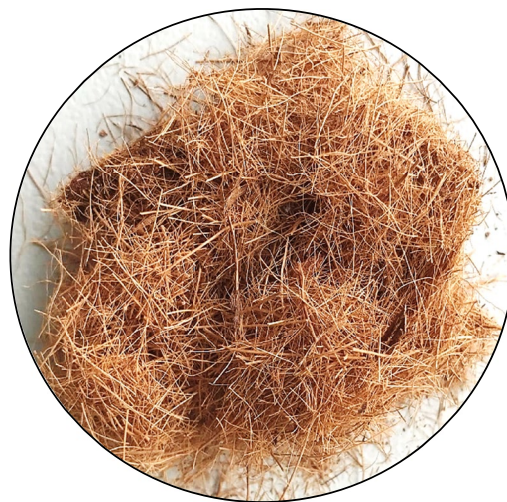
Fig. 1. Processed BF of 17 mm in length
