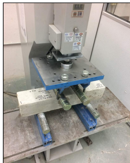
Fig. 4. Four point flexural test setup
