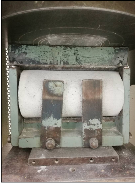
Fig. 5. Split tensile test setup
