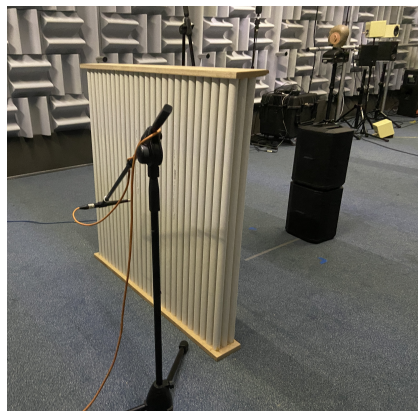
Fig. 7. Scheme of the laboratory stand for measuring IL: S – sound source; P_i – measurements points; h_S = 0.5 m; h_B = 1 m; d_M = 0.25 m; d_S = 1 m.
