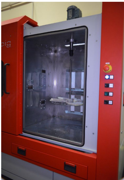
Fig. 1. View of the chamber of a microwave drier produced by Qbig
