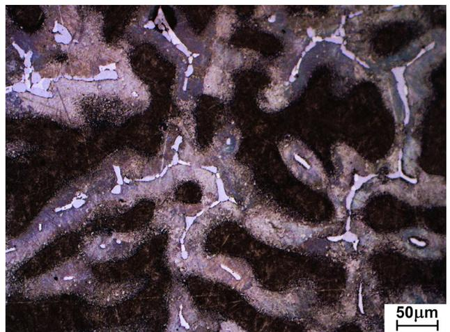
Fig. 6.5. Microstructure of ZnAl27Cu2 alloy cooling in the foundry gypsum mold, magnification 200x
