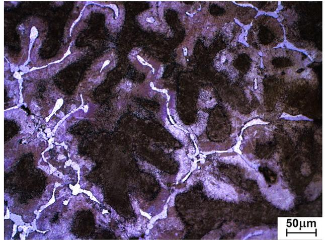
Fig. 6.4. Microstructure of ZnAl27Cu2 alloy cooling in the dried green sand mold, magnification 200x
