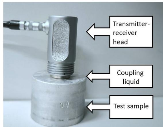
Fig. 3. Transmitter-receiver head on the tested sample
