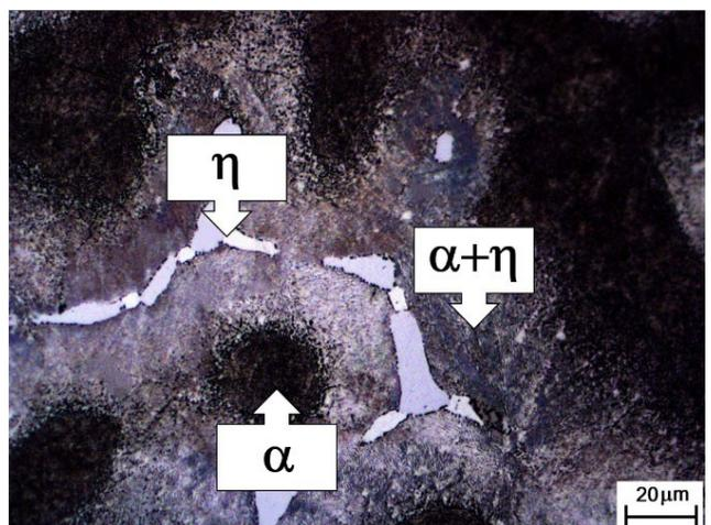
Fig. 7. Components of the microstructure of the ZnAl27Cu2 alloy poured into the casting gypsum mold, magnification 500x
