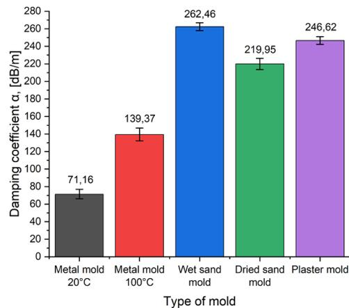
Fig. 5. Values of damping coefficient  $\alpha$  related to the cooling rate
