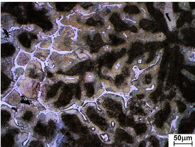
Fig. 6.3. Microstructure of ZnAl27Cu2 alloy cooling in the humid green sand mold, magnification 200x
