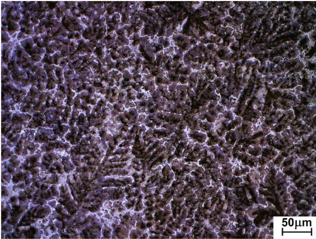
Fig. 6.1. Microstructure of ZnAl27Cu2 alloy cooling in the metal mold with an initial temperature of 20°C, magnification 200x
