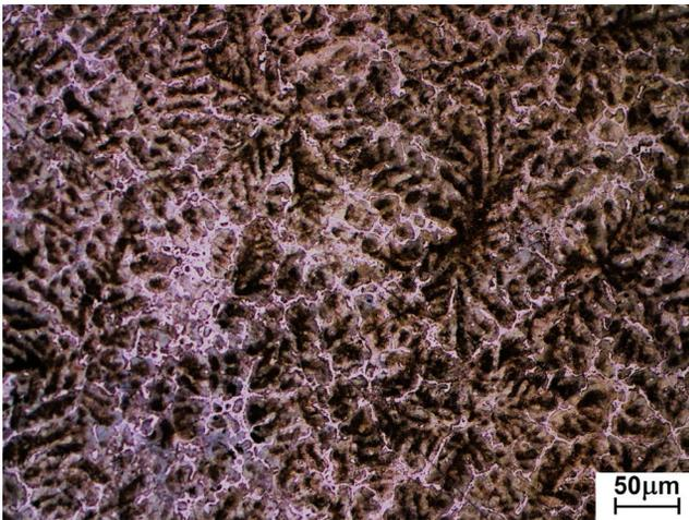
Fig. 6.2. Microstructure of ZnAl27Cu2 alloy cooling in the metal mold heated to the temperature of 100°C, magnification 200x
