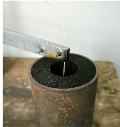
Fig. 2. The K-type thermocouple location in the mold
