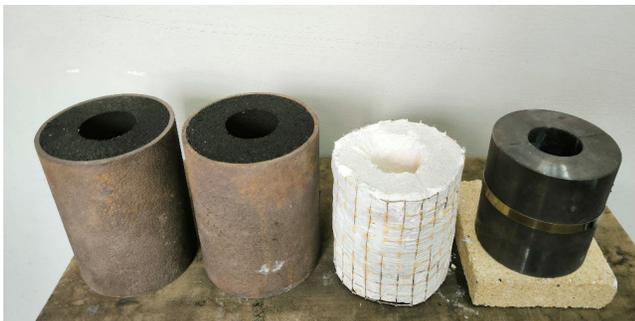
Fig. 1. Types of foundry mold used in the experiment: dry green sand mold, humid green sand mold, plaster mold, metal mold
