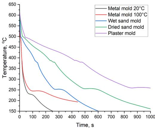
Fig. 4. Cooling curves of ZnAl<sub>27</sub>Cu<sub>2</sub> alloy
