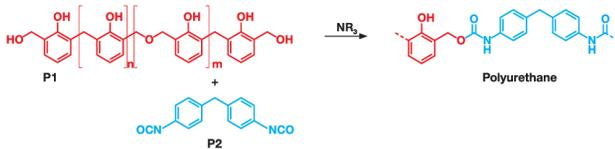
Fig. 1. Chemistry of the cold box binder system [29]
