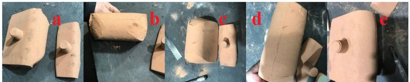
Fig. 4 Test casting cores produced using shooting machine parameters labeled a, b, c, d, e
