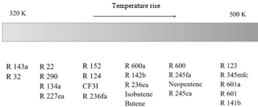
Fig. 2. Dependence of the working fluid selection on the temperature of the heat source
