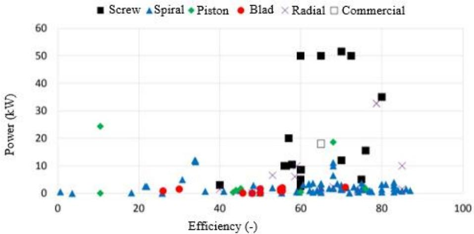
Fig. 6. “Coefficient of performance (COP)-power” expander experiment
