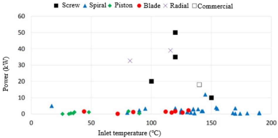
Fig. 4. “Temperature-power” expander experiment
