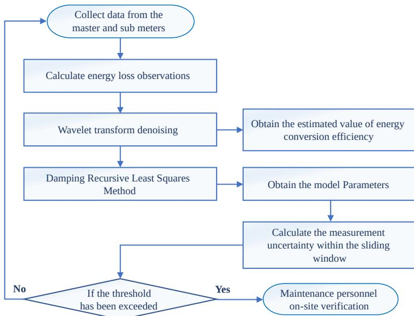
Fig. 2. Charging pile measurement performance analysis flowchart.
