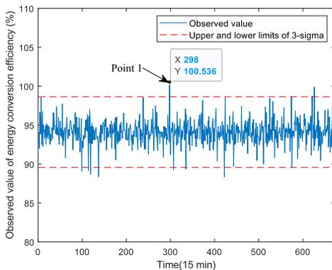
Fig. 4. Observation of energy conversion efficiency of the charging pile.
