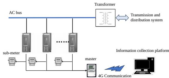
Fig. 1. Topology of electric vehicle charging pile.
