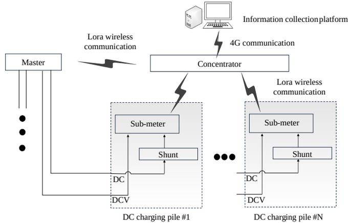
Fig. 3. Measurement and acquisition system.
