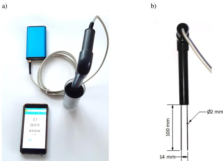
Fig. 2. a) Measurement setup, b) dimensions of the measuring probe.
