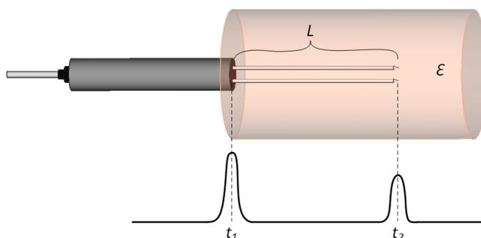
Fig. 1. Principle of TDR measurement in a medium with apparent dielectric permittivity  $\epsilon$ .  $L$  is the length of the probe,  $t_1$  and  $t_2$  are the recorded time of the pulse reflected from the beginning and the end of the probe rods, respectively.
