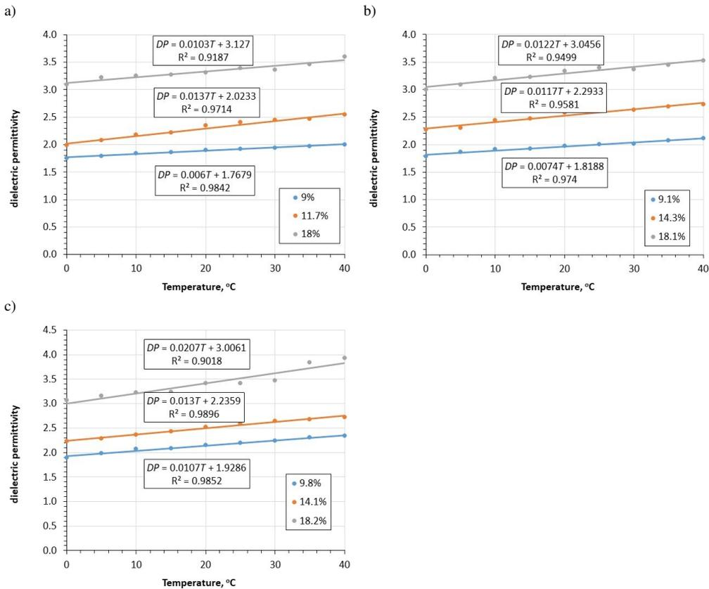
Fig. 5. Influence of temperature on dielectric permittivity for three levels of moisture content of three seed species: a) rapeseed, b) mustard, c) millet.
