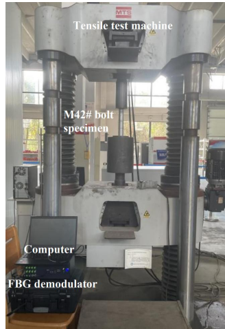
Fig. 8. The experimental setup for bolt crack detection.
