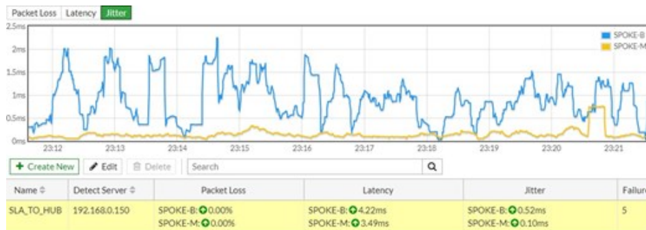
Fig. 18. Performance tunnel jitter FO-SDWAN
