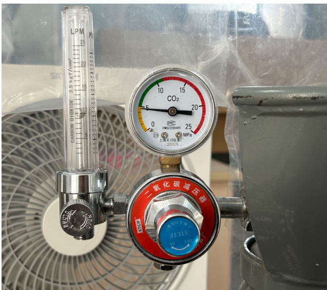
Fig. 11. CO 2 pressure reducing valve
