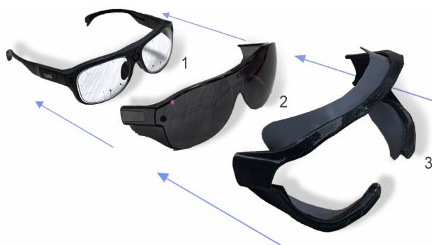
Fig. 3. Shield and its mounting mechanism (1 – eye-tracker; 2 – protective lens [25]; 3 – shield FV)
