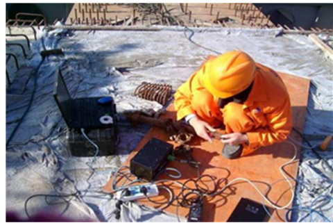
Fig. 15. On-site strain testing diagram
