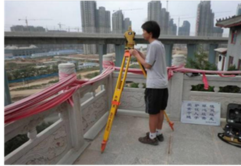
Fig. 18. On-site elevation measurement diagram
