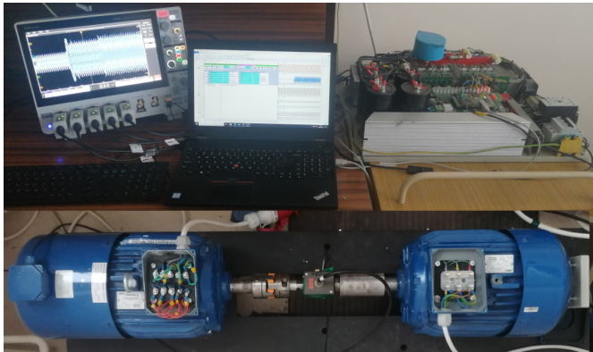
Fig. 12. Laboratory stand with five-phases induction motor (left) and induction motor emulated the load (right)
