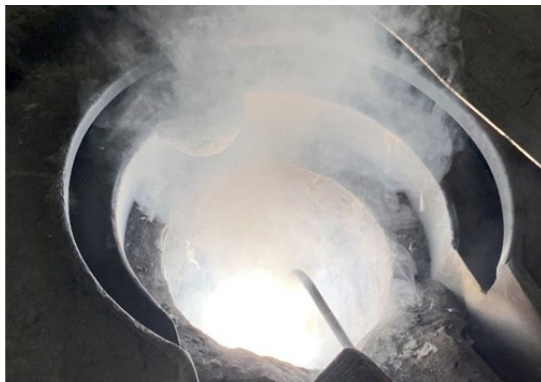
Fig. 5. Intensive evaporation of Mg from the melt
