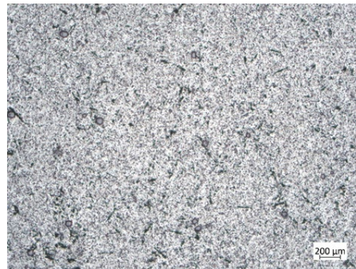
Fig. 6. Microstructure of AlB alloy (25x)
