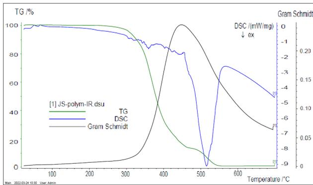
Fig. 2. Thermal analysis of the PolyCast™ material [3]
