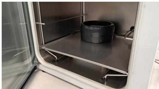
Fig. 6. View of the designed solenoid placed inside the incubator
