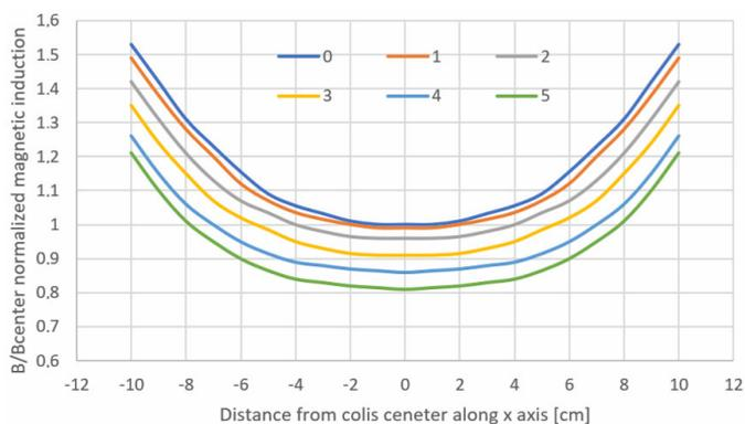
**Fig. 5.** Relative distribution of normalized magnetic induction  $B/B_{center}$  in the exposure coil along the horizontal  $x$ -axis and vertical  $y$ -axis (0, 1, 2, 3, 4, 5 –  $y$ -axis distance from the center point of the coil [cm])
