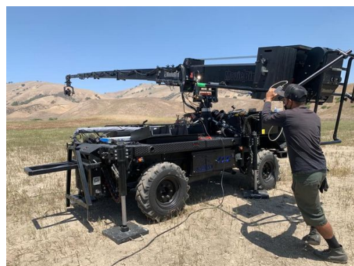
Fig. 1. MB45 telescopic camera crane arm in operation
