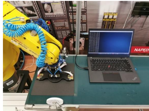
Fig. 11. Calibration process using the Fanuc LR Mate 200 robot
