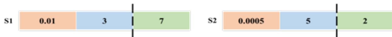
Fig. 3. Select crossover point between first and second fragment, or between second and third fragment
