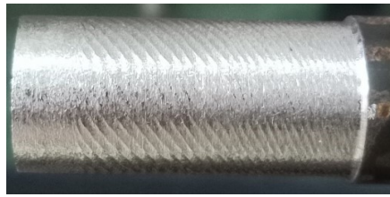
(b) Chatter imprinted on workpiece surface
