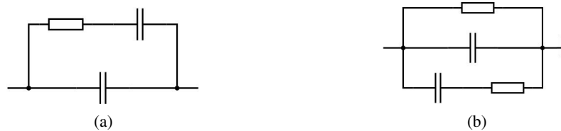
Fig. 6. Model of capacitive coupling between: two neighbouring coils (a); stator winding and machine housing (b)
