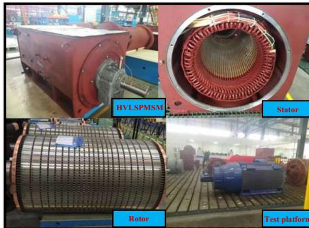
Fig. 2. Motor experiment platform
