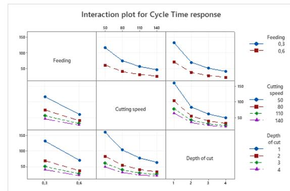
Fig. 6. Interaction plot effect for cycle time
