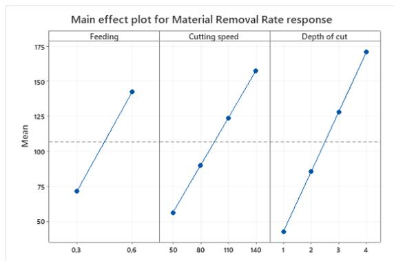
Fig. 7. Main plot effect for material removal rate
