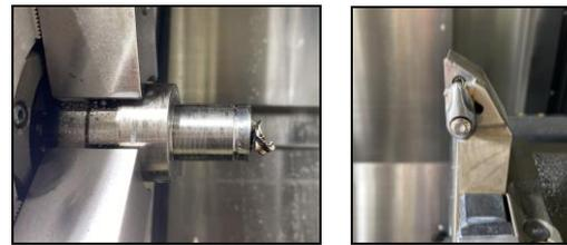
Fig. 11. Damaged materials and cutting tools in rank 1 and rank 2 parameter tests
