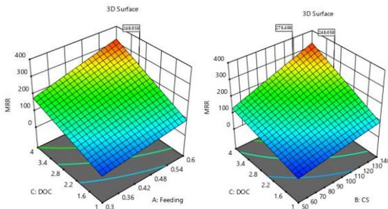
Fig. 14. Response surface for material removal rate
