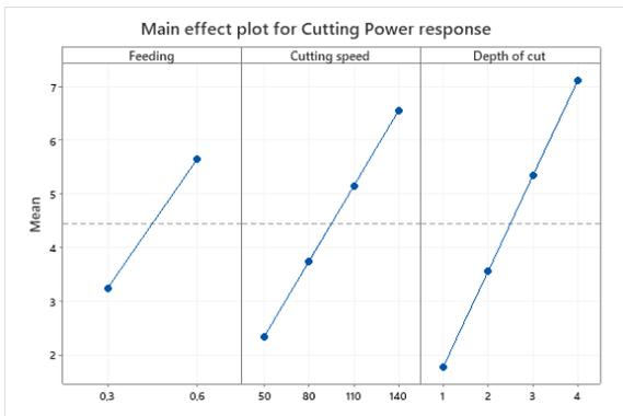
Fig. 9. Main plot effect for cutting power
