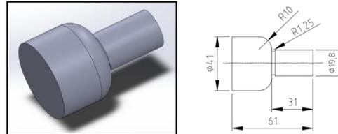
Fig. 2. Roughing dimensions and contours of yoke
