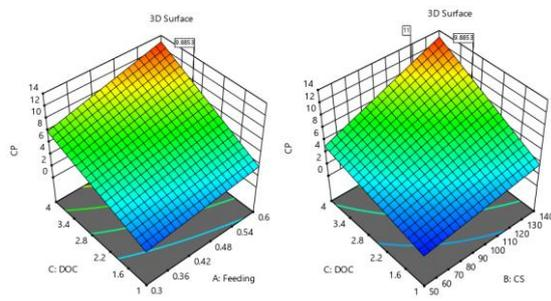
Fig. 15. Response surface for cutting power
