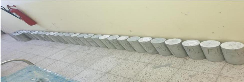
Fig. 10. Set of samples with random fiber distribution.
