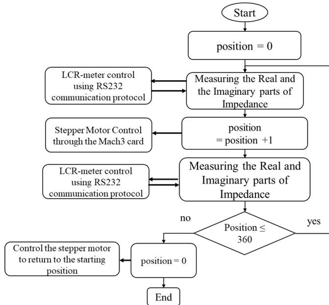
Fig. 3. Operation algorithm of the Eddy Current Non-Destructive scan system.
