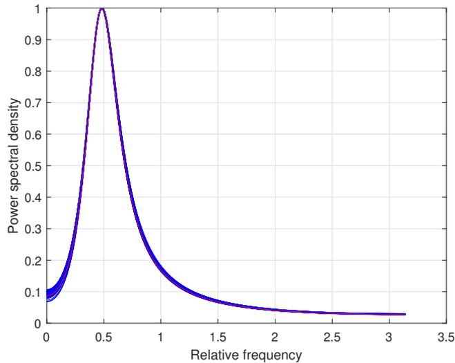
Figure 3: Normalized power spectral densities calculated from 100 identified models of ARMA time-series represented by binary-valued observations (blue lines) and the normalized pattern (red line) – random time-series decomposition,  $M = 2000$  and  $N = 512$
