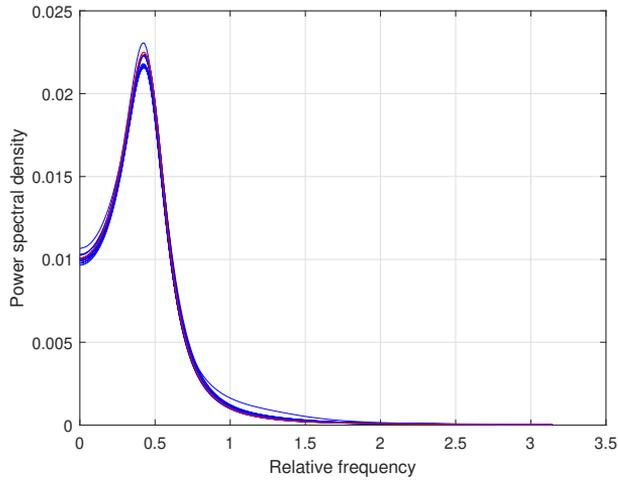
Figure 18: Power spectral densities calculated using 20 identified models of a normal-power Wiener time-series represented by quantized measurements (blue lines) and the pattern (red line) – power spectral density approximation,  $M = 2000$  and  $N = 512$
