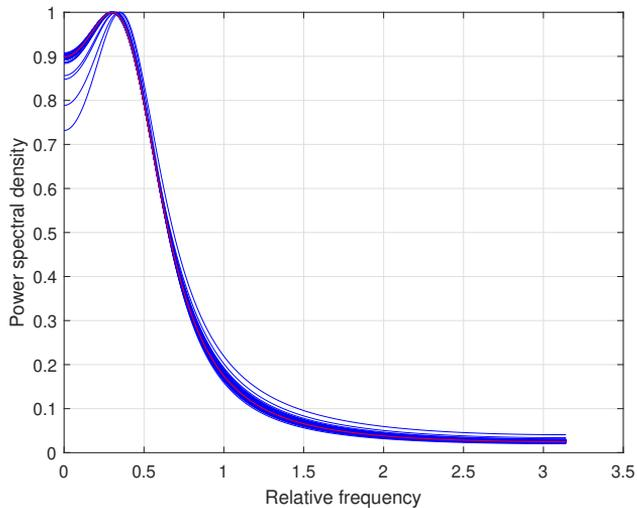
Figure 21: Power spectral densities calculated using 100 identified models of a high-power ARMA time-series represented by quantized measurements (blue lines) and the pattern (red line) – random time-series decomposition,  $M = 10000$  and  $N = 1024$
