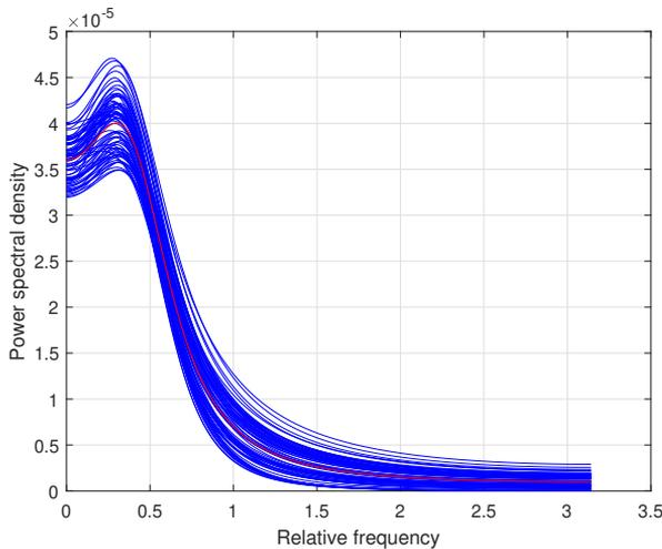
Figure 15: Power spectral densities calculated using 75 identified models of ultra low-power ARMA time-series represented by quantized measurements (blue lines) and the pattern (red line) – random time-series decomposition,  $M = 1000$  and  $N = 256$
