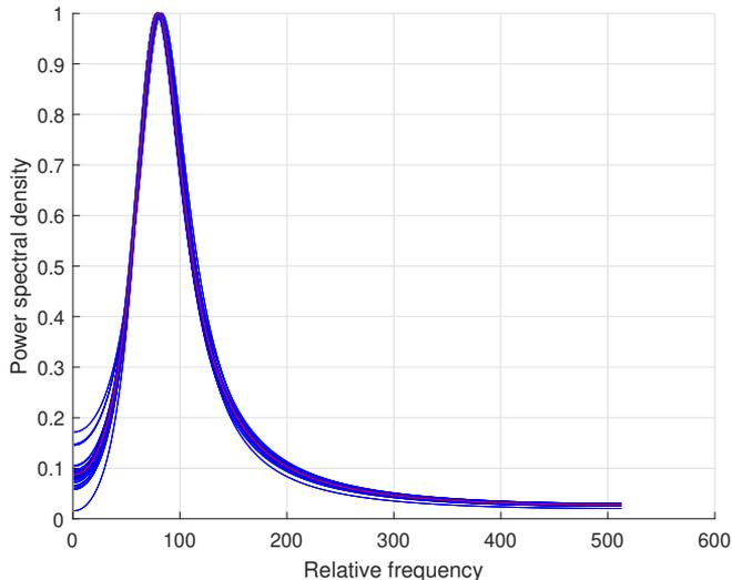
Figure 5: Normalized power spectral densities calculated from 100 identified models of ARMA time-series represented by binary-valued observations (blue lines) and the normalized pattern (red line) – direct power spectral density approximation,  $M = 2000$  and  $N = 128$
