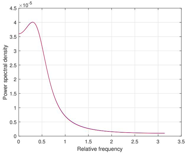
Figure 16: Mean value of 75 power spectral densities calculated from identified models of ultra low-power ARMA time-series represented by quantized measurements (blue line) and the pattern (red line) – random time-series decomposition,  $M = 1000$  and  $N = 256$
