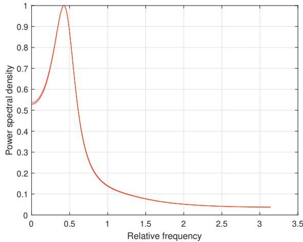
Figure 10: Normalized mean value of 10 power spectral densities calculated from identified Wiener models for the corresponding simulated time-series represented by binary-valued observations (blue line) and the normalized pattern (red line) – direct power spectral density approximation,  $M = 2000$  and  $N = 128$
