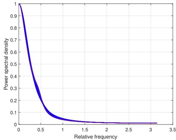
Figure 12: Normalized power spectral densities calculated using 50 identified Wiener–Hammerstein models for the corresponding time-series represented by binary-valued observations (blue lines) and the normalized pattern (red line) – direct power spectral density approximation,  $M = 2000$  and  $N = 512$
