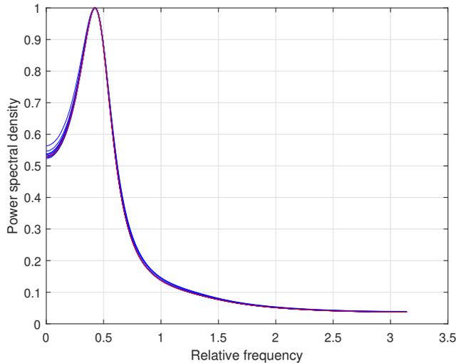
Figure 9: Normalized power spectral densities calculated using 10 identified Wiener models for the corresponding time-series represented by binary-valued observations (blue lines) and the normalized pattern (red line) – direct power spectral density approximation,  $M = 2000$  and  $N = 512$
