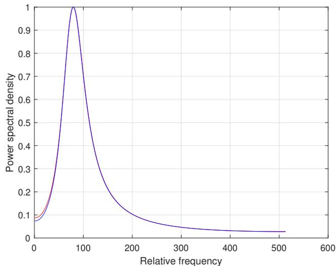
Figure 6: Mean value of 100 normalized power spectral densities calculated from identified models of ARMA time-series represented by binary-valued observations (blue line) and the normalized pattern (red line) – direct power spectral density approximation,  $M = 2000$  and  $N = 128$
