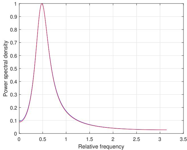
Figure 2: Normalized mean value of 100 power spectral densities calculated from identified models of ARMA time-series represented by binary-valued observations (blue line) and the normalized pattern (red line) – random time-series decomposition,  $M = 2000$  and  $N = 512$
