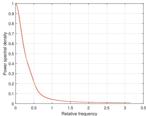
Figure 13: Normalized mean value of 50 power spectral densities calculated from the identified Wiener–Hammerstein models using the corresponding simulated time-series represented by binary-valued observations (blue line) and the normalized pattern (red line) – direct power spectral density approximation,  $M = 2000$  and  $N = 512$
