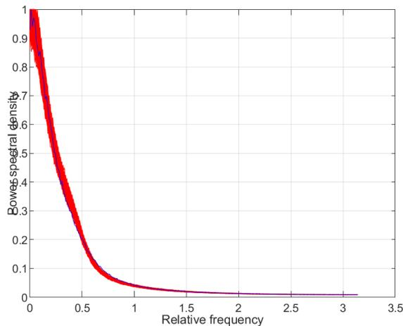
Figure 11: Normalized averaged periodograms calculated using 10000 realizations of binary-valued observations obtained using the simulated Wiener–Hammerstein model (red lines) and the normalized averaged periodogram of a single realization of binary-valued observations obtained using the recovered Wiener–Hammerstein model (blue line) – direct power spectral density approximation,  $M = 2000$  and  $N = 512$
