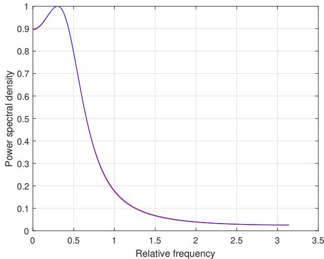
Figure 23: Mean value of 100 power spectral densities calculated from identified models of a high-power ARMA time-series represented by quantized measurements (blue line) and the pattern (red line) – random time-series decomposition,  $M = 10000$  and  $N = 1024$
