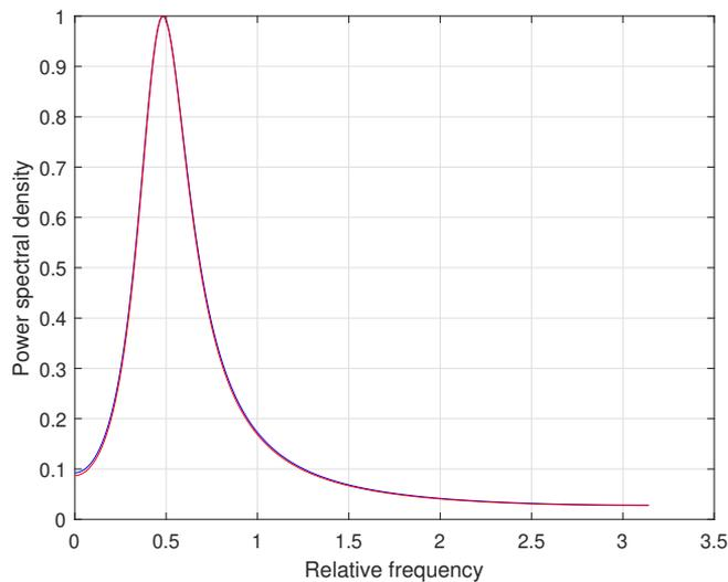
Figure 4: Mean value of 100 normalized power spectral densities calculated from identified models of ARMA time-series represented by binary-valued observations (blue line) and the normalized pattern (red line) – random time-series decomposition,  $M = 2000$  and  $N = 512$
