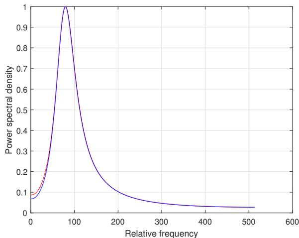
Figure 8: Normalized mean value of 100 power spectral densities calculated from identified models of ARMA time-series represented by binary-valued observations (blue line) and the normalized pattern (red line) – direct autocorrelation function approximation,  $M = 2000$  and  $N = 128$
