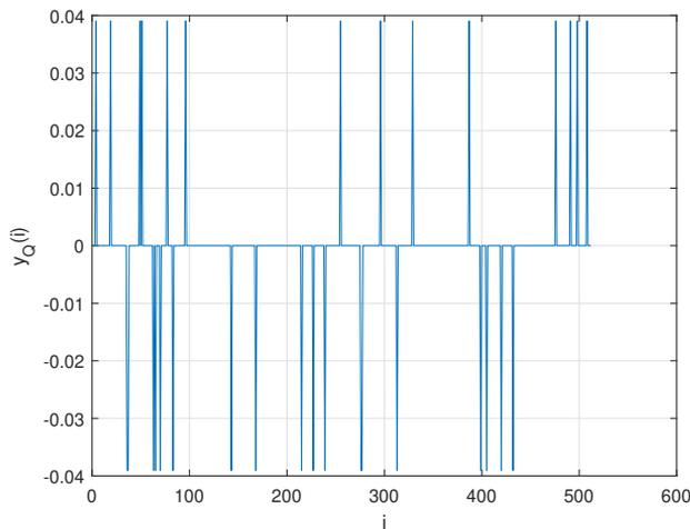
Figure 14: Exemplary 512-sample of quantized measurements acquired from an ultra low-power ARMA time-series realization
