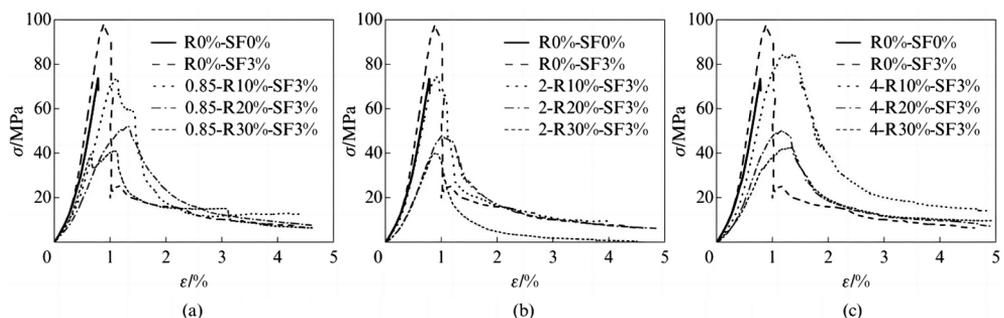
Fig. 6. Stress-strain curves of UHSRC specimens under three kinds of rubber particle sizes [22]:
