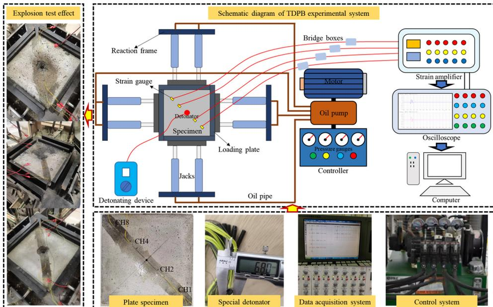
Fig. 3. Central explosion tests of RCC plate specimens
