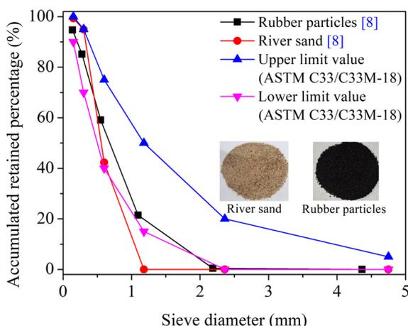
Fig. 2. The grain size distribution curves of the river sand and rubber particles for the test [8]
