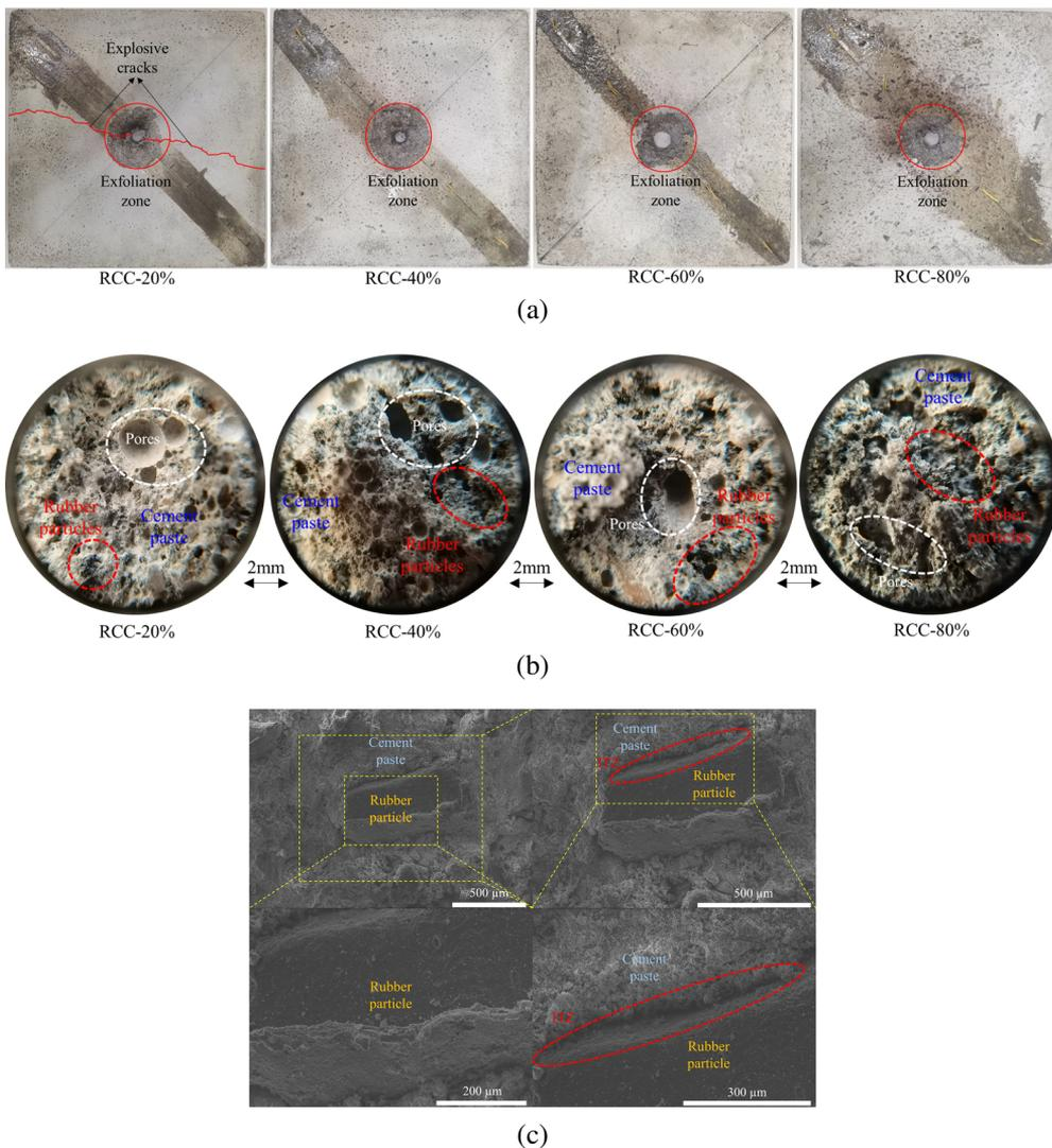
Fig. 5. Macro-damage states of explosion in the center of RCC plate specimens and meso-fracture morphology: (a) Macroscopic damage states, (b) Meso-fracture morphology (OM), (c) Meso-fracture morphology (SEM)
