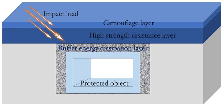
Fig. 1. Schematic diagram of a typical multi-level underground protective structure
