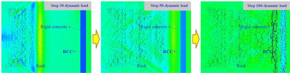
Fig. 8. Numerical simulation test of explosion shock wave action for multi-level protective structure
