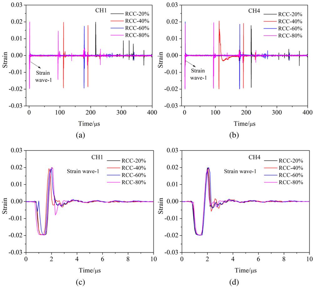
Fig. 4. Propagation characteristics of strain waves in central explosion tests of RCC plate specimens: (a) CH1-strain waves, (b) CH4-strain waves, (c) CH1-strain wave-1, (d) CH4-strain wave-1
