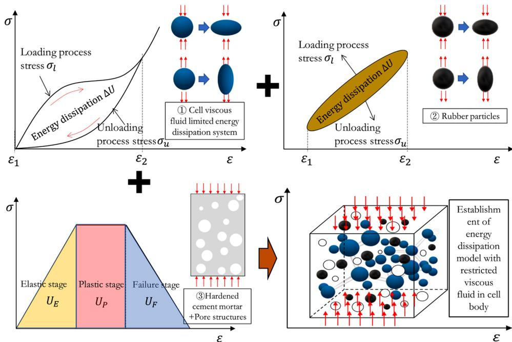
Fig. 9. Schematic diagram of energy dissipation model with restricted viscous fluid in cell body of MCVFRCEAM
