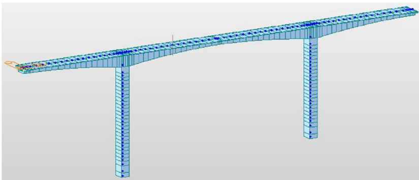
Fig. 4. Three-dimensional model for finite element analysis
