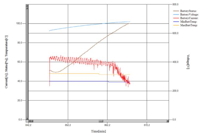
**Fig.7.** Time window corresponding to a single collection taken from the group of collections representing catenary mode and charging state at initial SOC value of 50%
