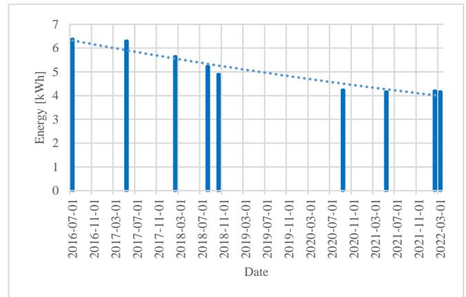
**Fig.10.** Energy delivered to the battery at SOC criterion:  $SOC \in <71\%, 100\%$
