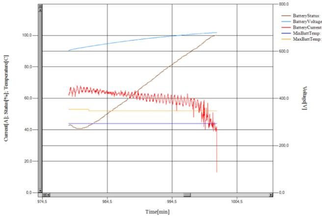
**Fig.8.** Time window corresponding to a single collection taken from the group of collections representing catenary mode and charging state at initial SOC value of 44%
