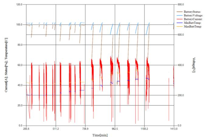
**Fig.6.** Waveforms of selected collections in "GroupCatenaryCharge": Battery status, Battery voltage, Battery current, Min battery temperature, Max battery temperature
