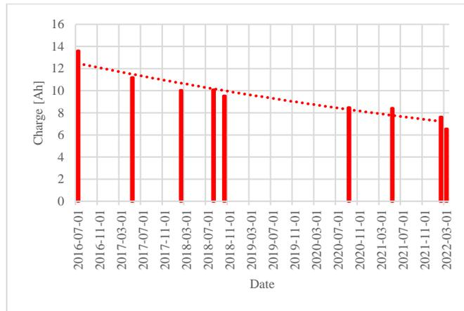
**Fig.11.** Charge delivered to the battery at Voltage criterion:  $U_{batt} \in <643$  V, 680 V>
