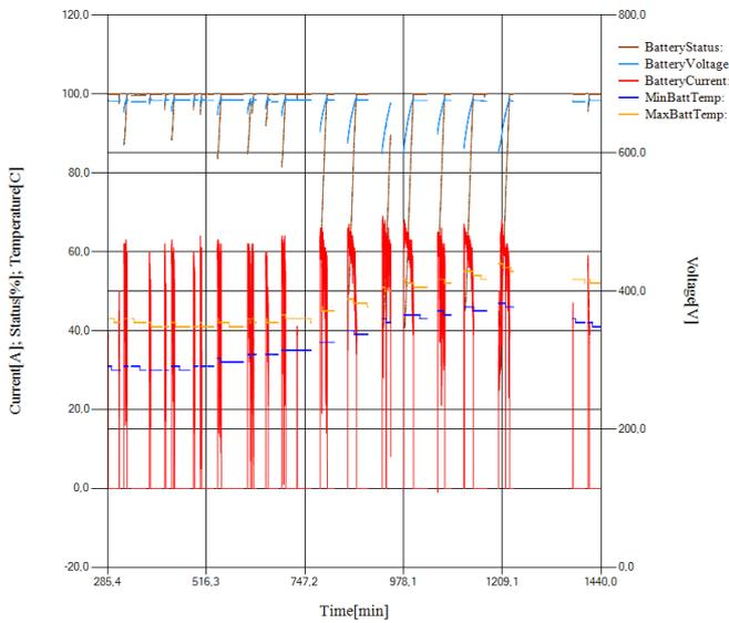
**Fig.4.** Waveforms of selected group collections in catenary mode: Battery status, Battery voltage, Battery current, Min battery temperature, Max battery temperature
