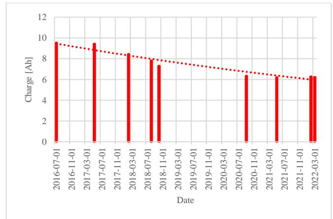
**Fig.9.** Charge delivered to the battery at SOC criterion:  $SOC \in <71\%, 100\%$
