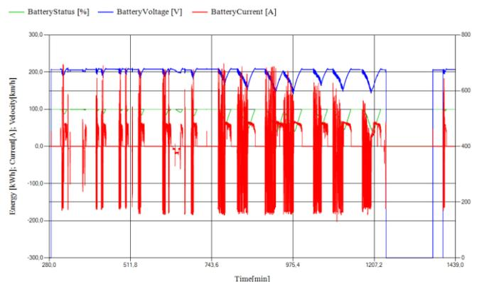
**Fig.3.** Waveforms of selected trolleybus per-one day data: battery status, battery voltage, and battery current
