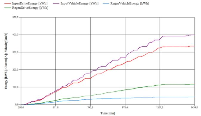
**Fig.1.** Waveforms of selected trolleybus per-one day data: input drive energy (red), input vehicle energy (purple), regenerative vehicle energy (blue), regenerative drive energy (green)
