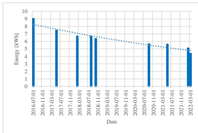
**Fig.12.** Energy delivered to the battery at Voltage criterion:  $U_{batt} \in <643$  V, 680 V>
