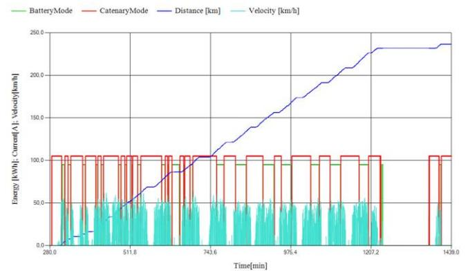
**Fig.2.** Waveforms of selected trolleybus per-one day data: battery mode of operation (green), catenary mode of operation (red), distance travelled by the vehicle (blue), velocity (green)
