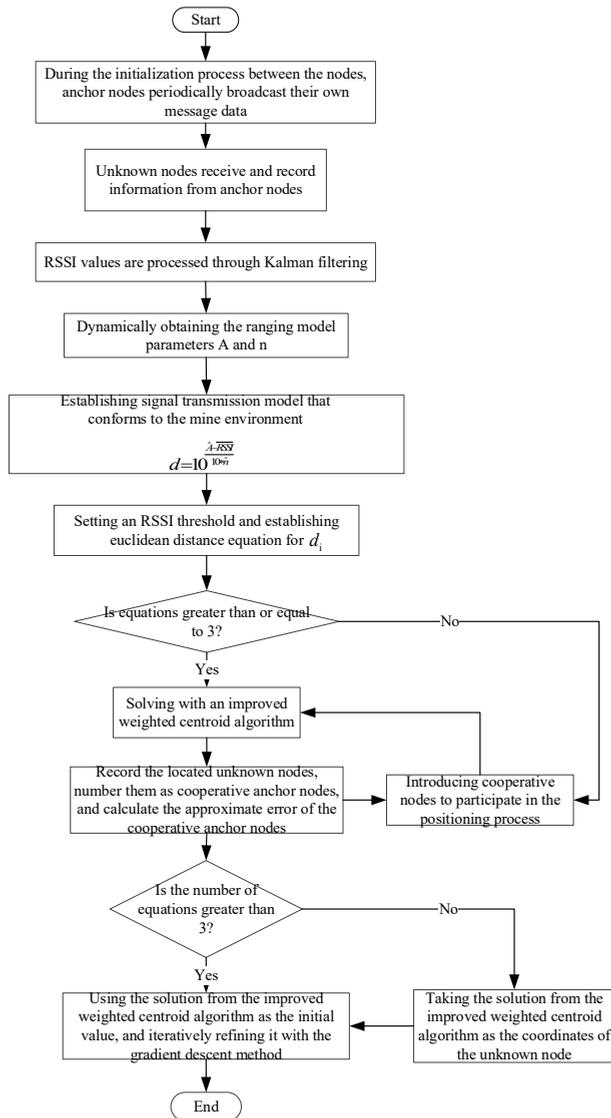
Fig. 4. Flowchart for the implementation of the positioning algorithm
