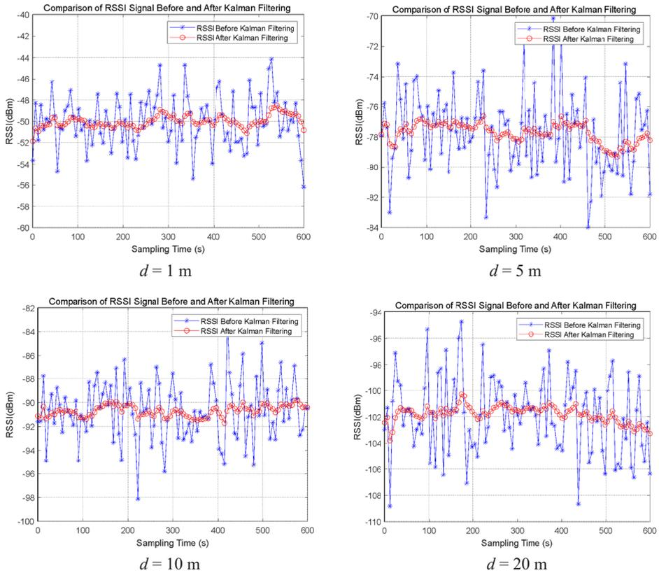
Fig. 1. Comparison of *RSSI* Signal before and After Kalman Filtering
