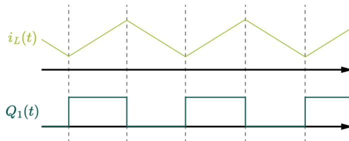
Fig. 2. Generic current waveform of a switching converter
