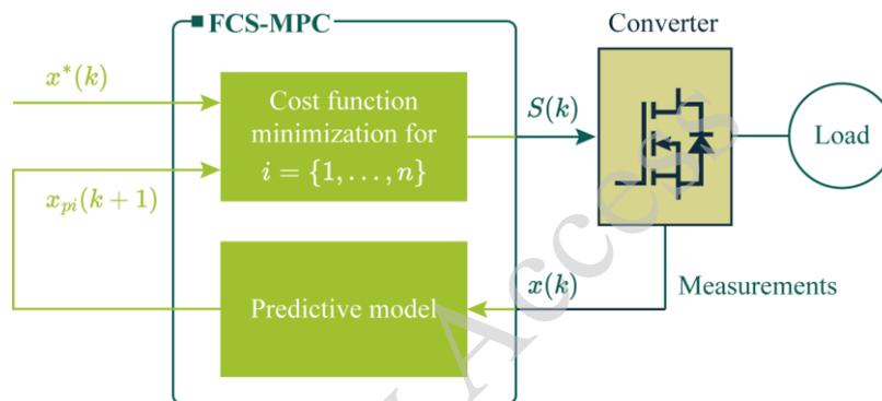
Fig. 5. Generic control diagram of FCS-MPC
