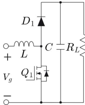
Fig. 1. Boost converter diagram
