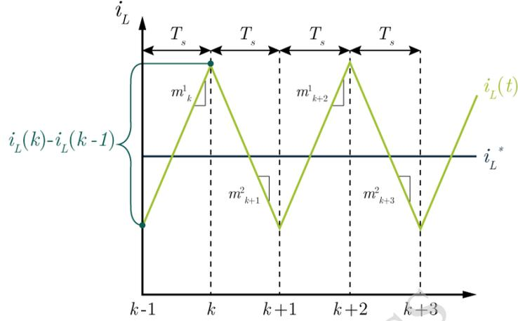
Fig. 3. Inductor current waveform under MF-PC based on inductor current averaging
