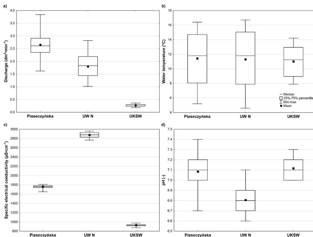
Fig. 2. Distribution of measured values of: a) spring discharge, b) water temperature, c) specific electrical conductivity, d) pH in the three investigated springs in the period from June 2023 to May 2024; source: own study
