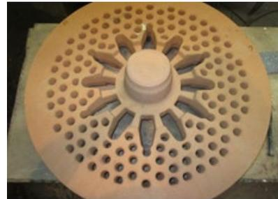
Fig. 7. Produced core for casting – RC brake disc made using cold-box-amine technology with Surwaybest additive
