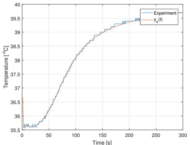
**Fig. 3.** The comparison of the step responses model vs experiment for  $N = 8$ . Sensor 1 - top, sensor 2 - middle, sensor 3 - bottom.
