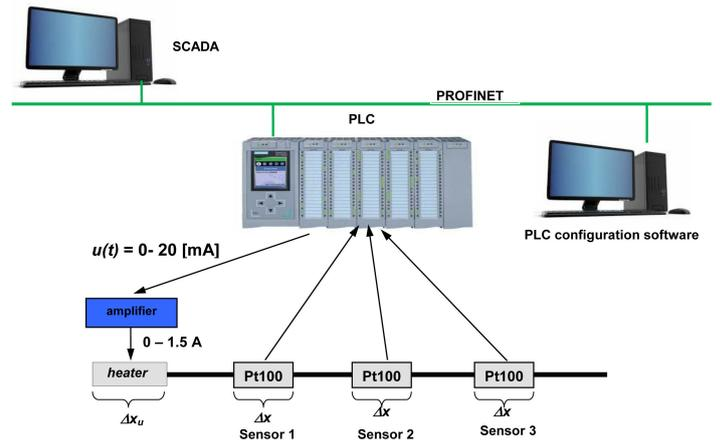
Fig. 1. The experimental system.
