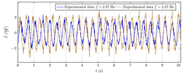
**Fig. 10.** Experimental data for acceleration of pendulation of the PTMD
