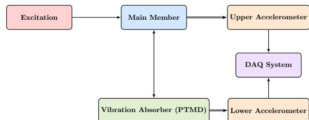
Fig. 5. Scheme of the measuring system used during the experimental tests
