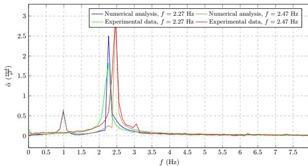
**Fig. 12.** Comparative spectral analysis for the numerical and experimental model
