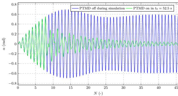
**Fig. 14.** Amplitude of pendulation (angular displacement) of the main pendulum member  $\alpha(t)$  under the influence of varying activation time
