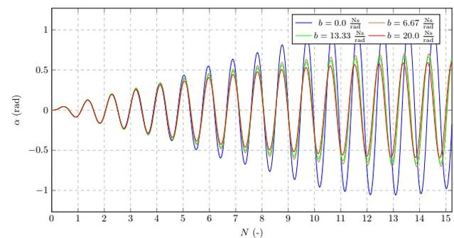
**Fig. 13.** Pendulation of the main member of the double pendulum under the influence of various damping coefficient values - direct comparison
