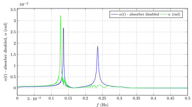
Fig. 21. Sweep frequency analysis in spectral domain - angular displacement  $\alpha(t)$  amplitude values - impact of absorber activation in 700s
