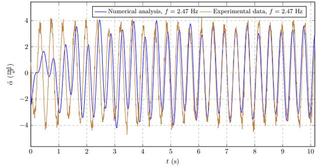
**Fig. 9.** Comparative results for acceleration of pendulation of the main member of double pendulum for excitation frequency 2.47 Hz
