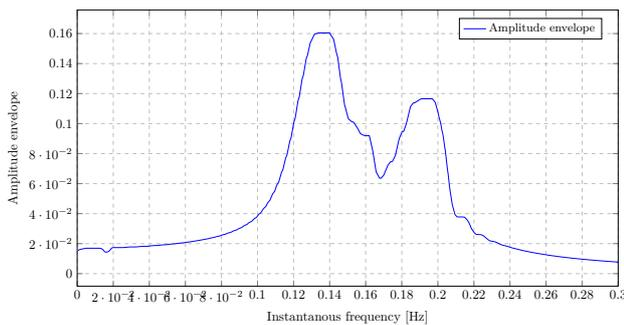
Fig. 23. Amplitude of vibration of  $\alpha(t)$  while sweeping the excitation frequency
