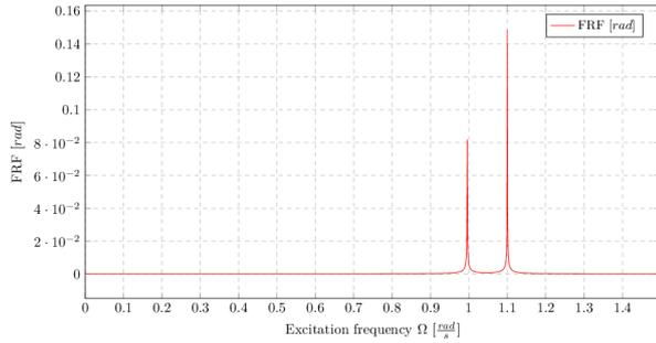
Fig. 22. PTMD frequency response function
