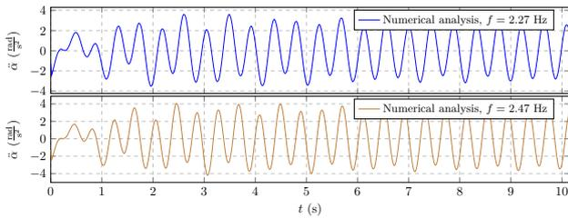
**Fig. 7.** Validation analysis for acceleration of pendulation of the main member of double pendulum
