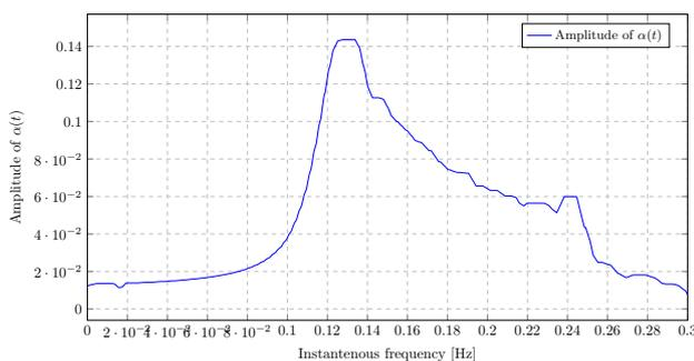
Fig. 24. Amplitude of vibration of  $\alpha(t)$  while sweeping the excitation frequency and PTMD device attached to the system
