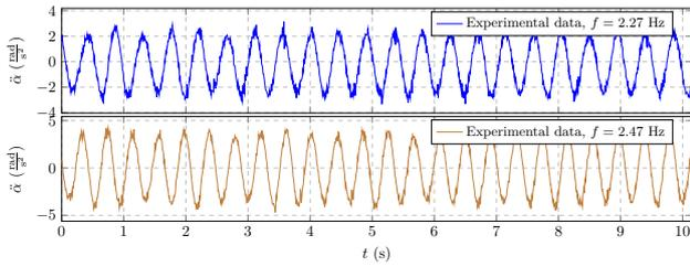
**Fig. 6.** Experimental data for acceleration of pendulation of the main member of double pendulum
