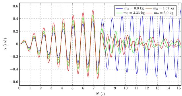
**Fig. 15.** Pendulation of the main member of the double pendulum in dependence on various masses of the transferred liquid - direct comparison
