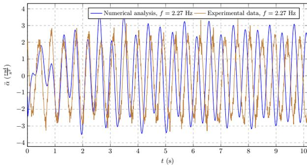
**Fig. 8.** Comparative results for acceleration of pendulation of the main member of double pendulum for excitation frequency 2.27 Hz
