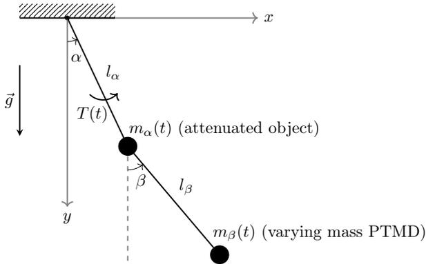
**Fig. 1.** Scheme of a mathematical double pendulum - a simplified model adopted in the analysis
