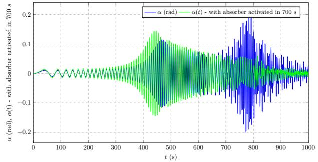
Fig. 20. Sweep frequency analysis - angular displacement  $\alpha(t)$  amplitude values - impact of absorber activation in 700s
