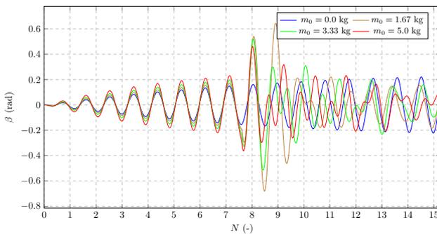
Fig. 16. Pendulation of the second member of the double pendulum in dependence on various masses of the transferred liquid - direct comparison
