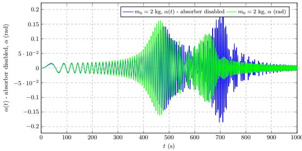
Fig. 18. Sweep frequency analysis - angular displacement  $\alpha(t)$  amplitude values for the system with and without PTMD
