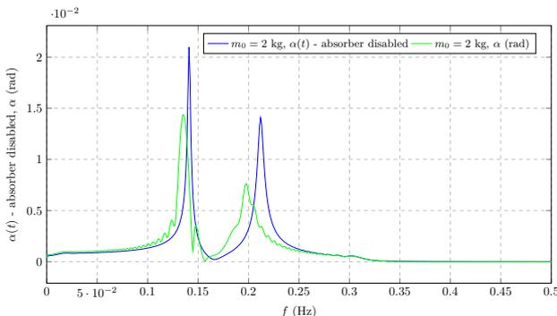
Fig. 19. Sweep frequency analysis in spectral domain - angular displacement  $\alpha(t)$  amplitude values for the system with and without PTMD
