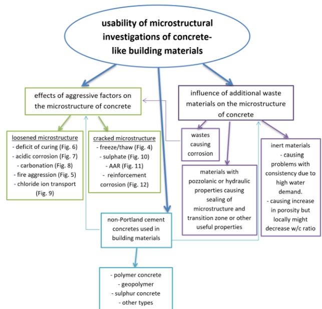
**Figure 3.** Usability of microstructural investigations of concrete-like building materials
