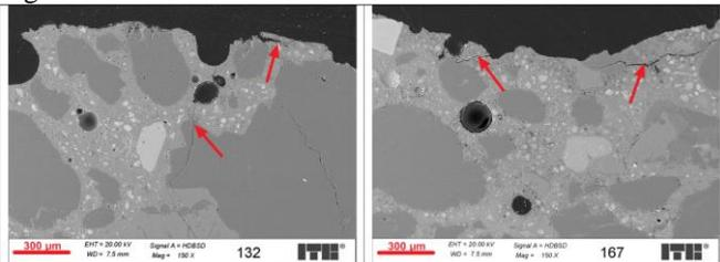
**Figure 8.** Effects of carbonation on the microstructure of concrete (arrows mark degraded areas)
