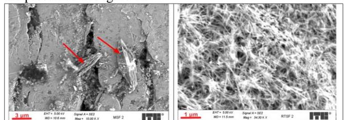
**Figure 12.** Surface of steel reinforcement received from corroded concrete (arrows mark products of corrosion)
