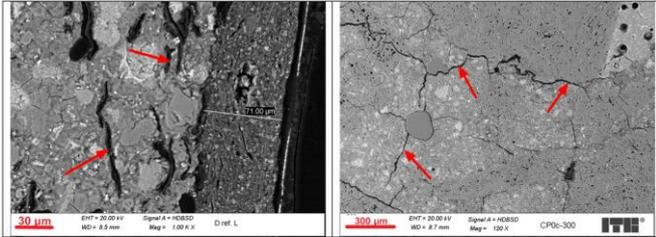
**Figure 5.** Effects of fire aggression on the microstructure of concrete (arrows mark cracks in microstructure) [20]
