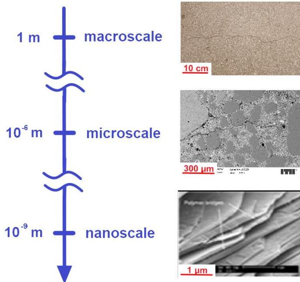
**Figure 2.** Structural level in building materials engineering ([8], updated)
