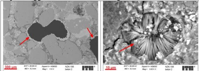
**Figure 10.** Effects of sulphate aggression on the microstructure of concrete (arrows mark degraded areas)
