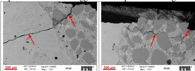
Figure 4. Effects of freeze/thaw on the microstructure of concrete (arrows mark degraded areas)
