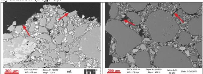
**Figure 6.** Effects of deficit in curing on the microstructure of concrete (arrows mark degraded areas)
