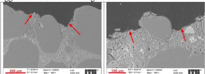
**Figure 9.** Effects of chloride ion transport on the microstructure of concrete (arrows mark degraded areas)
