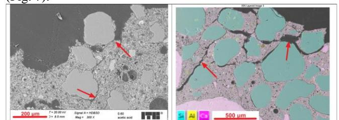
**Figure 7.** Effects of acidic aggression on the microstructure of concrete (arrows mark degraded areas)
