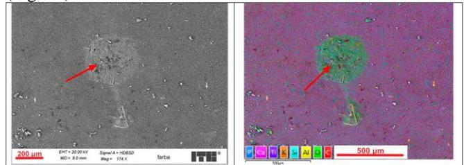
**Figure 11.** Effects of alkali-aggregate reaction on the microstructure of concrete (arrows mark degraded areas)
