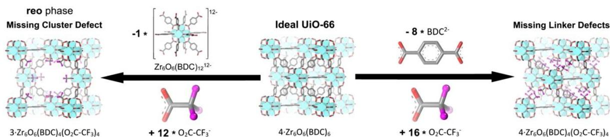
Figure 9. Diagram illustrating the structure and composition differences between ideal and defective UiO-66 unit cells (Shearer et al., 2016).
