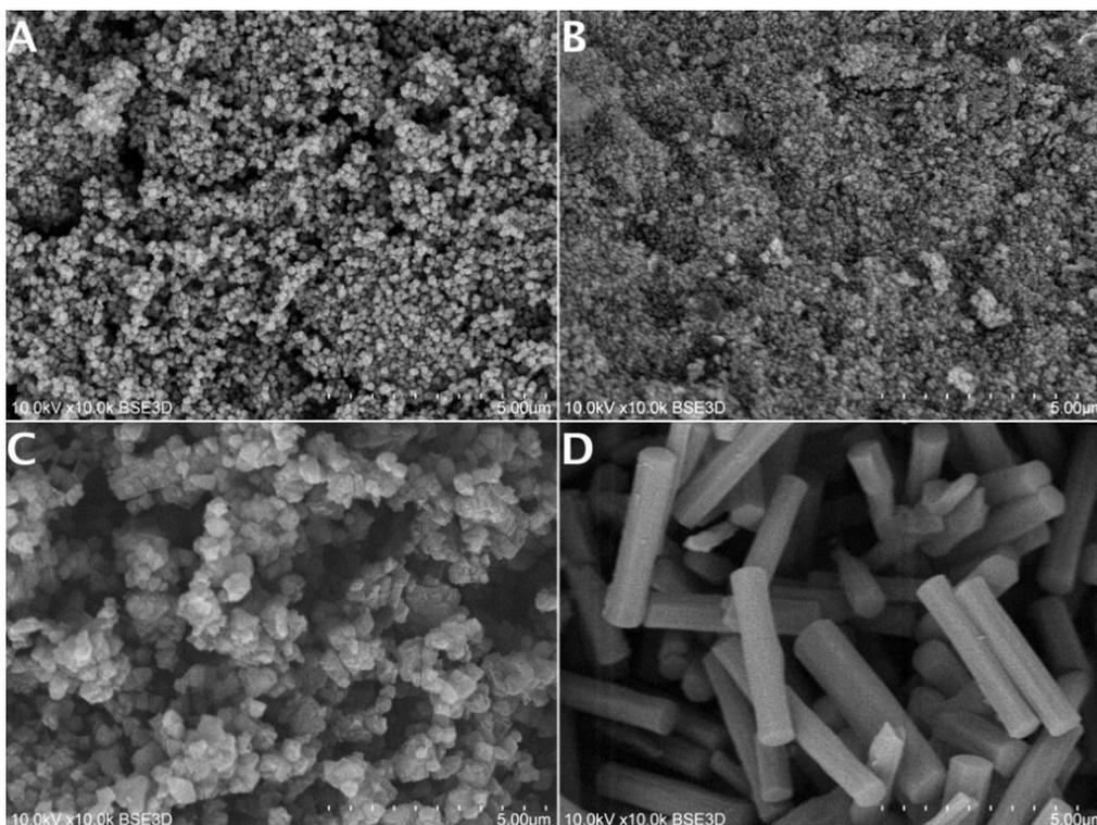
Figure 8. SEM microphotographs of composites acriflavine@MOF: ACF@MOF-808 (A), ACF@UiO-66 (B), ACF@UiO-67 (C), ACF@NU-(D) (Jodłowski et al., 2022).
