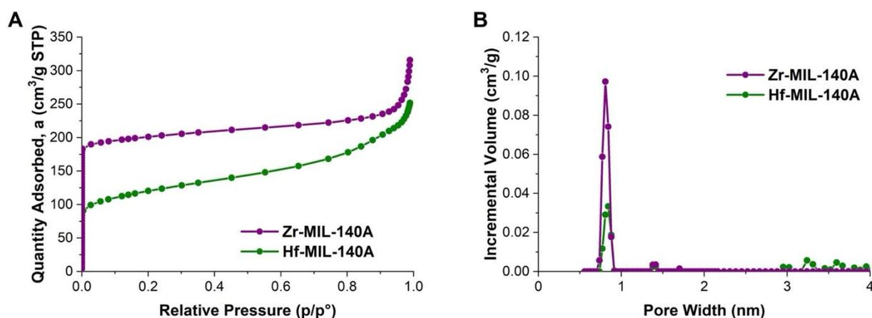
Figure 7.  $N_2$  adsorption isotherms (A) and DFT pore size distribution of MIL-140A samples (B) (Jodłowski, Kurowski, et al., 2023).
