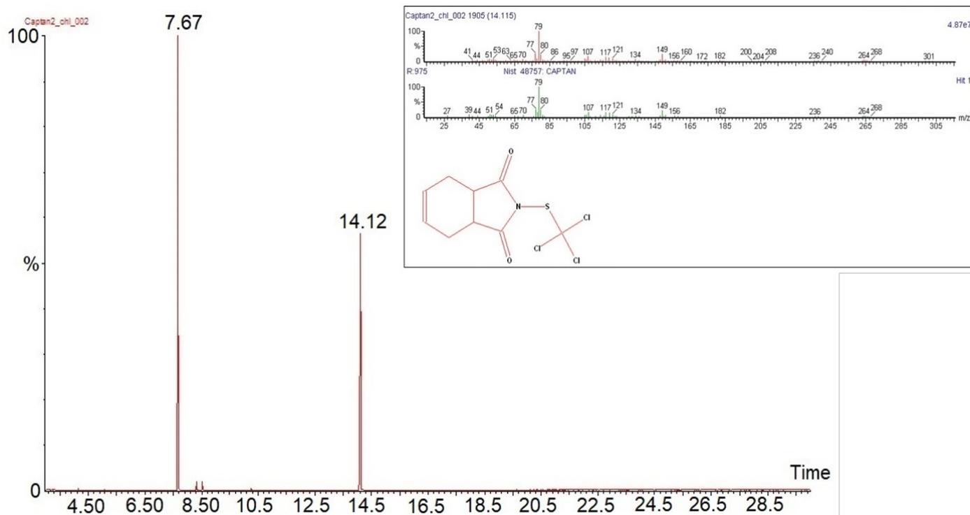
Fig. 2. Chromatogram of captan (retention time 14.12 min) in *n*-hexane extract; tetradecane as the internal standard at 7.67 min with mass spectrum of captan determined in NIST database.
