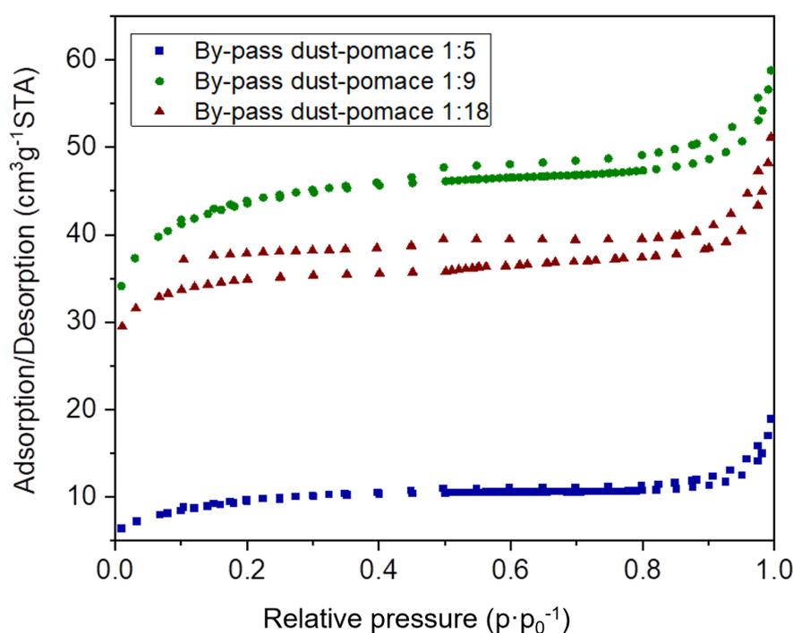
**Fig. 4.** Adsorption-desorption isotherms for the mineral-carbonaceous materials with different initial substrate ratios.
