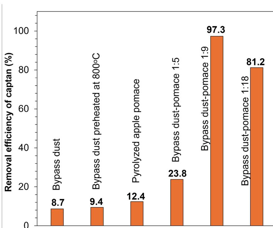
Fig. 6. Removal efficiency of captan v/s different materials.
