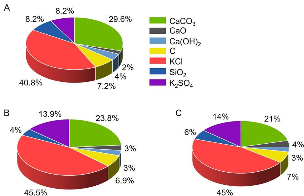
**Fig. 3.** Mineral composition of: A – bypass dust, B – bypass dust preheated at 500°C, C – bypass dust preheated at 800°C, determined by X-ray diffraction (XRD).
