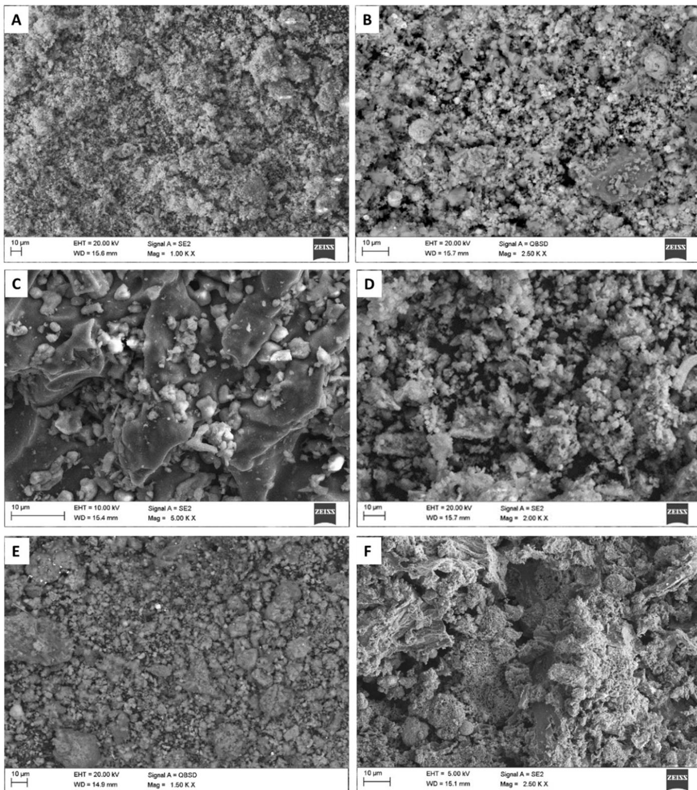
**Fig. 5.** SEM images: A – bypass dust, B – bypass dust preheated at 800°C, C – apple pomace pyrolyzed at 800°C, D – bypass dust-pomace ratio 1:5 pyrolyzed at 800°C, E – bypass dust-pomace ratio 1:9 pyrolyzed at 800°C, F – bypass dust-pomace ratio 1:18 pyrolyzed at 800°C.
