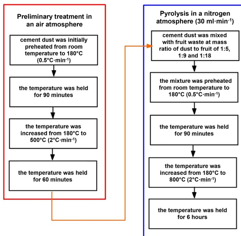
Fig. 1. Step by step synthesis of mineral-carbonaceous materials.
