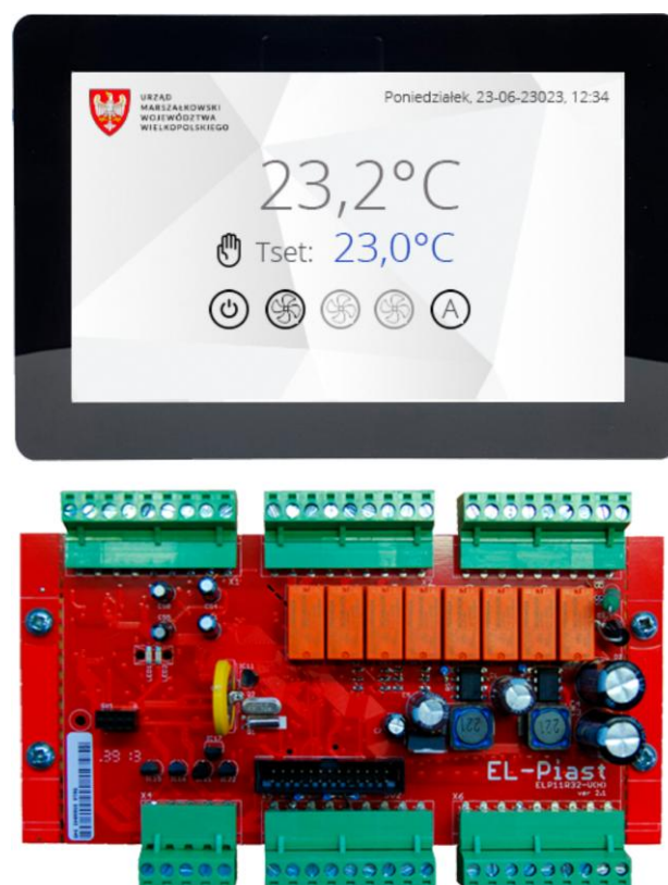
Fig.11. A set of room automation devices designed for measuring, setting the temperature and regulating the operation of the air handling unit. The PLC controller is located in the power supply and control cabinet together with other automation components necessary for the operation of air conditioning and ventilation. The operator panel is located on the wall of the office rooms.
