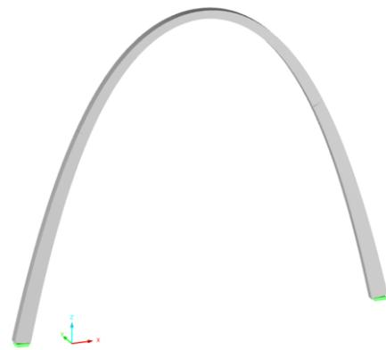
Fig.10. The final design of the reinforced concrete arch
