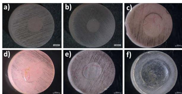
**Fig. 5.** Optical microscopy images of the structure of the surface layer in the defect of discs from: a) ProBase Hot Pink, b) Vertex Rapid Simplified, c) ProBase Cold Polymer Pink, d) Vertex Self Curing, e) Villacryl SP V4, f) Premacryl Plus
