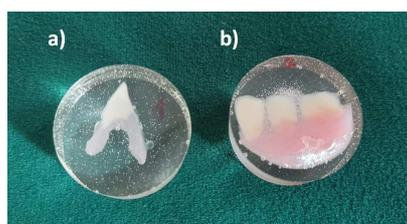
**Fig.3.** Fragments of the denture intended for testing: a) structure obtained by cutting with a plane perpendicular to the mandibular arch, b) structure obtained by cutting with a plane tangential to the mandibular arch
