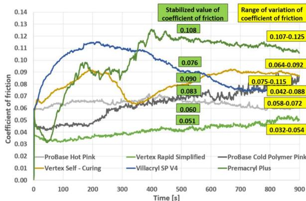
Fig. 10. Sliding friction coefficients of acrylic polymers in artificial saliva
