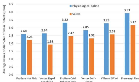
**Fig.11.** Wear resistance in sliding friction of acrylic resins on denture plates, in the presence of physiological saline and artificial saliva
