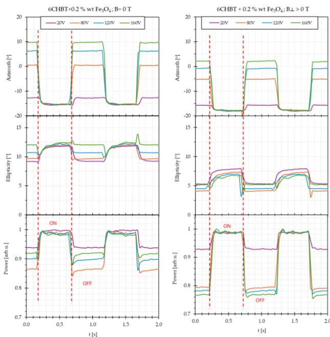
Fig.4. The azimuth and ellipticity values, corresponding to the applied steering voltages ranging from 20 to 160 V, were obtained for LC cells filled with 6CHBT + 0.2 wt%  $\text{Fe}_3\text{O}_4$ : a) without a magnetic field; b) with the applied magnetic field.
