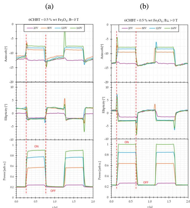
Fig.5. The azimuth and ellipticity values, corresponding to the applied steering voltages ranging from 20 to 160 V, were obtained for LC cells filled with 6CHBT + 0.5 wt%  $\text{Fe}_3\text{O}_4$ : a) without a magnetic field; b) with the applied magnetic field.
