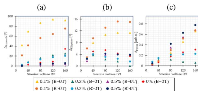
Fig. 6. Switching range of a) azimuth, b) ellipticity, and c) power under electric and magnetic fields as a function of the wt% concentration of MNPs
