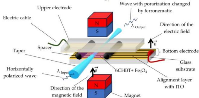
Fig. 1. Polarization measurement setup: scheme of the LC cell filled 6CHBT+Fe<sub>3</sub>O<sub>4</sub>.
