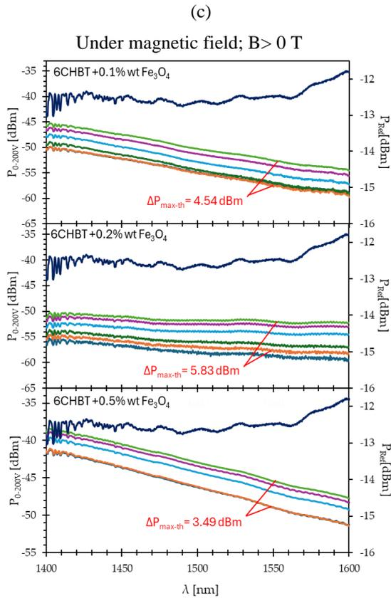
Fig.2. Transmission spectra were obtained for the LC cell filled with a) pure LC without a magnetic field and b) ferronematic with different wt. concentration of  $\text{Fe}_3\text{O}_4$  - 0.1%; 0.2%; 0.5% without magnetic field; and c) ferronematic with different wt. concentration of  $\text{Fe}_3\text{O}_4$  - 0.1%; 0.2%; 0.5% with magnetic field.
