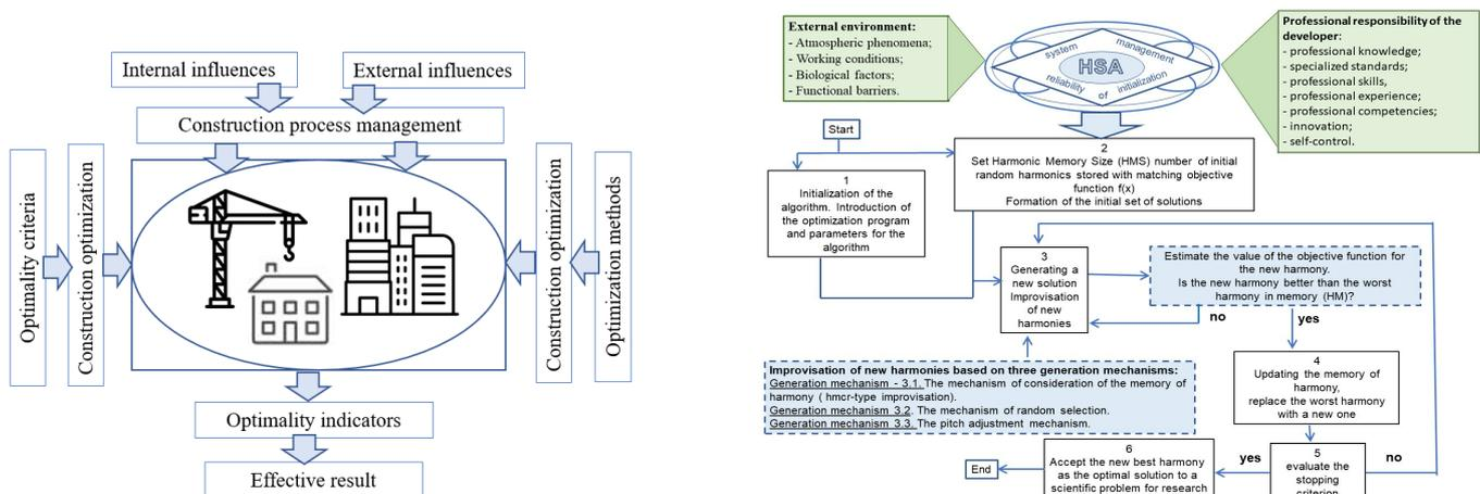
Fig.1. Implementation of optimization methods in construction (left) and modification of the harmony search algorithm using the system management model (right) (source own findings based on [11, 12])
