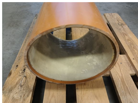
Fig. 8. Composite structure – PVC pipe + CIPP liner
