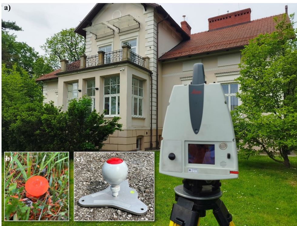
Fig. 2. Survey components; a) laser scanner, b) control point, c) reference sphere
