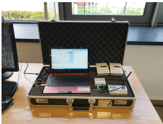
Fig. 3. iBros remote sensors set measuring CO 2
