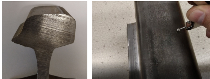
Fig. 4. Measurement of rail head profile and manual guidance of the measuring tip [Photo. J. Kukulski]
