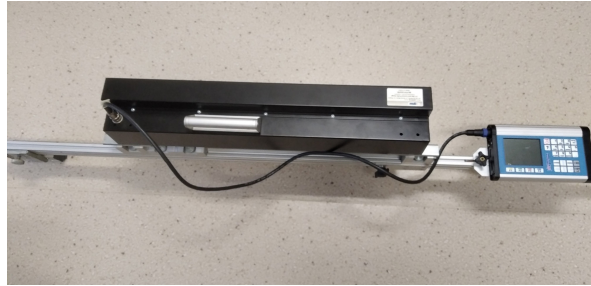
Fig. 3. X-Y profiler measuring system [Photo. J. Kukulski]
