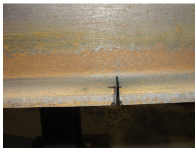
Fig. 5. Damage to the bottom flange – full-depth notch
