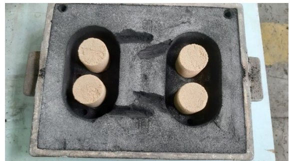
Fig. 2. The prepared drag of the mould with the placed specimens
